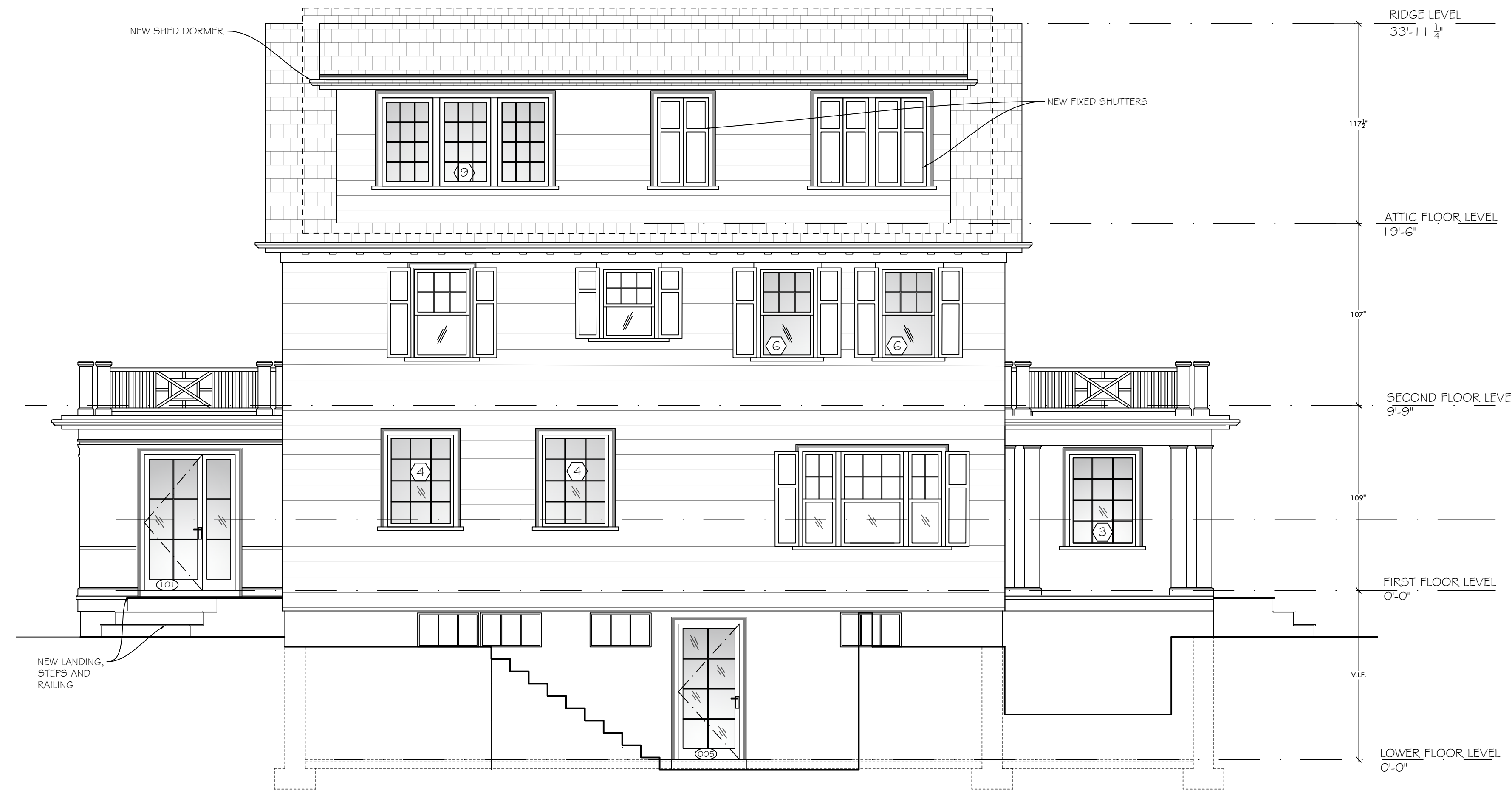
PROPOSED REAR ELEVATION DEMOLITION Scale: 1/4" = 1'-0"
