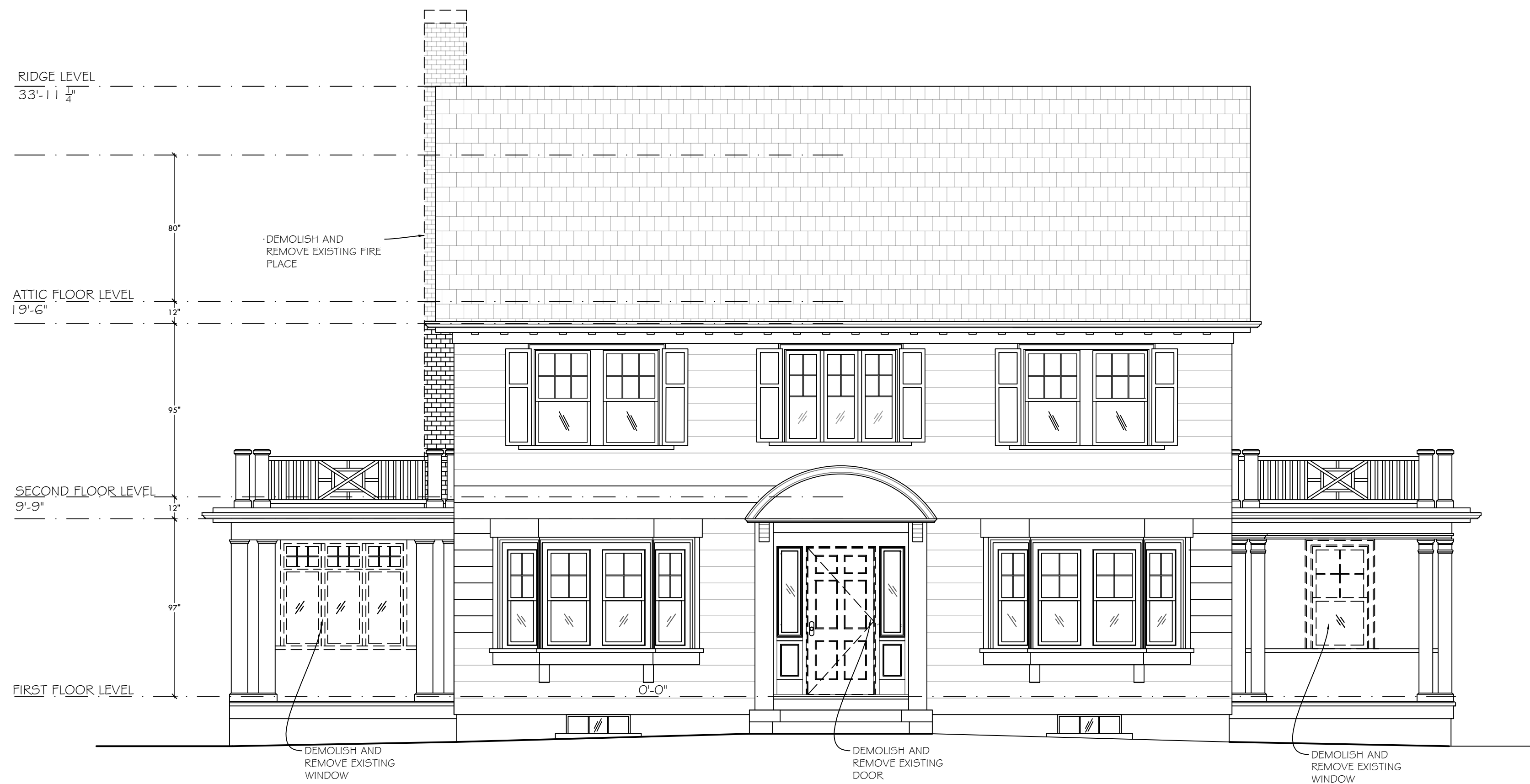
FRONT ELEVATION- DEMOLITION SCALE: 1/4" = 1'-0"
