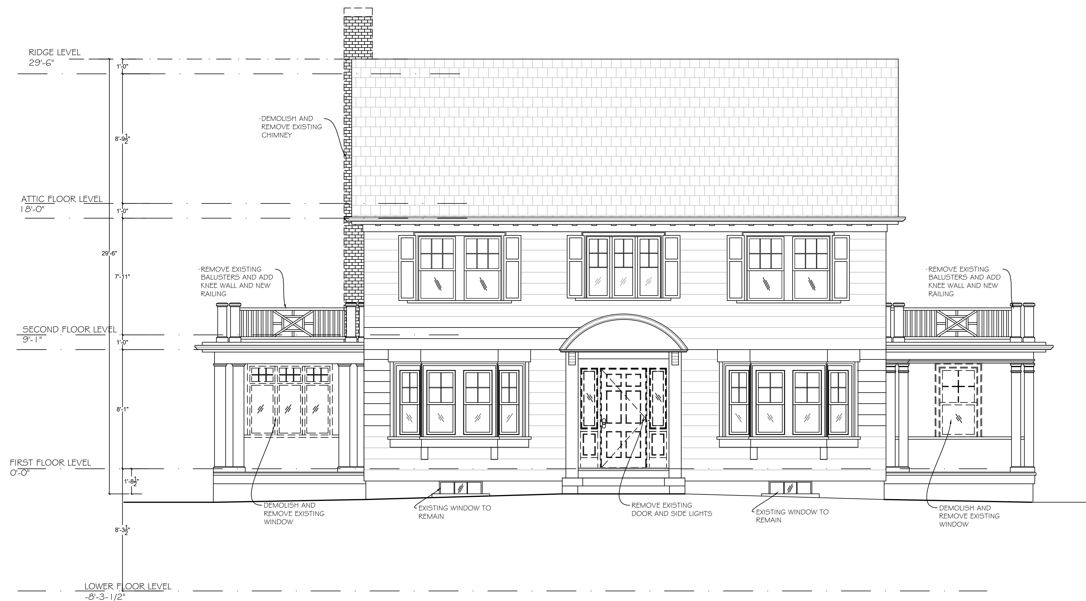
FRONT ELEVATION- DEMOLITION SCALE: 1/4" = 1'-0"
