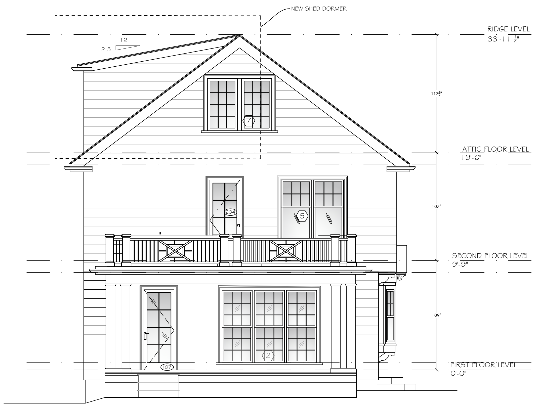
PROPOSED LEFT ELEVATION Scale: 1/4" = 1'-0"
