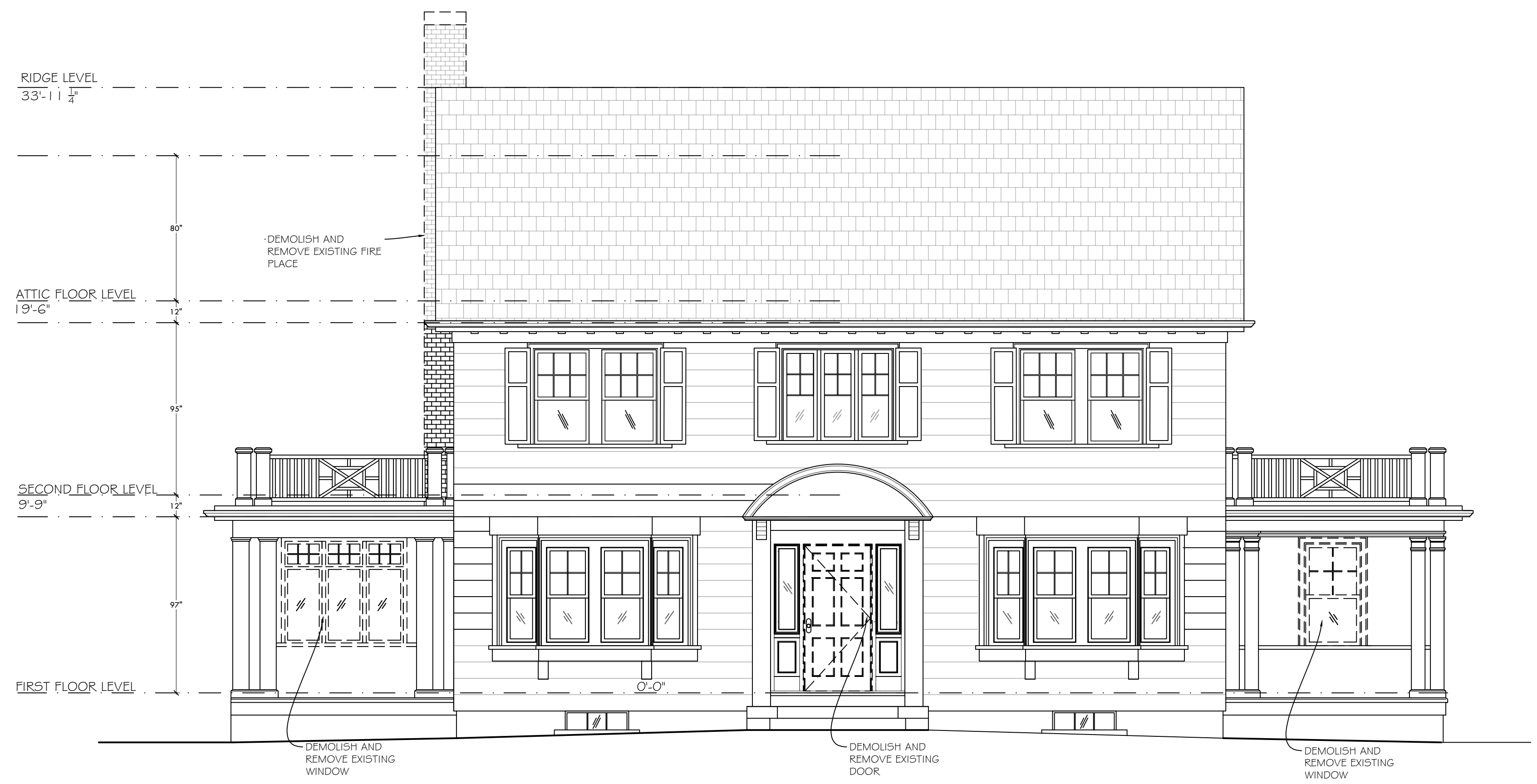
FRONT ELEVATION- DEMOLITION SCALE: 1/4" = 1'-0"
