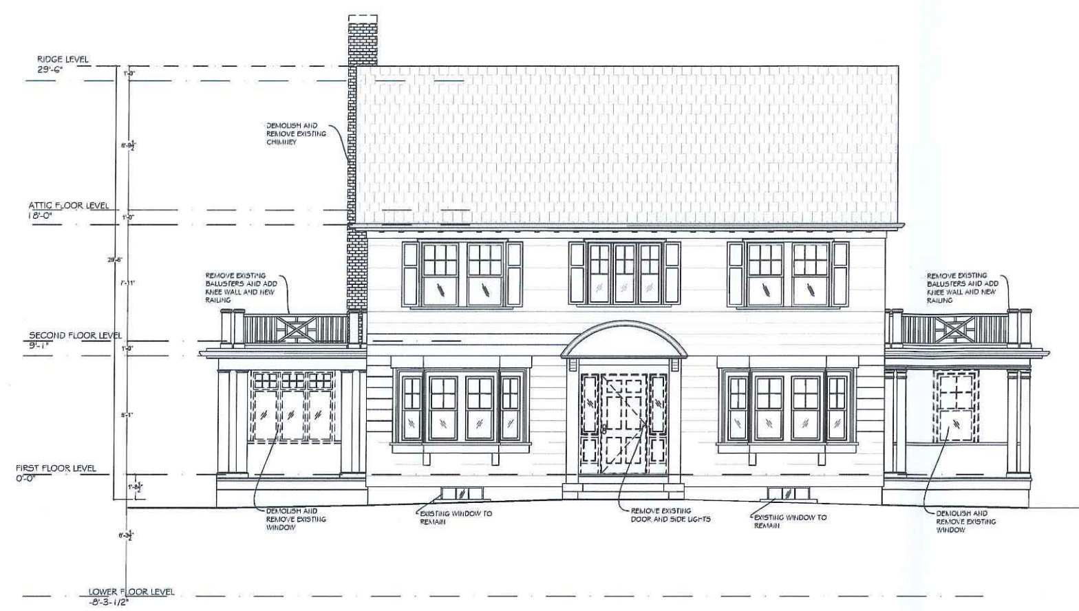
FRONT ELEVATION- DEMOLITION SCALE: 1/4" = 1'-0"
