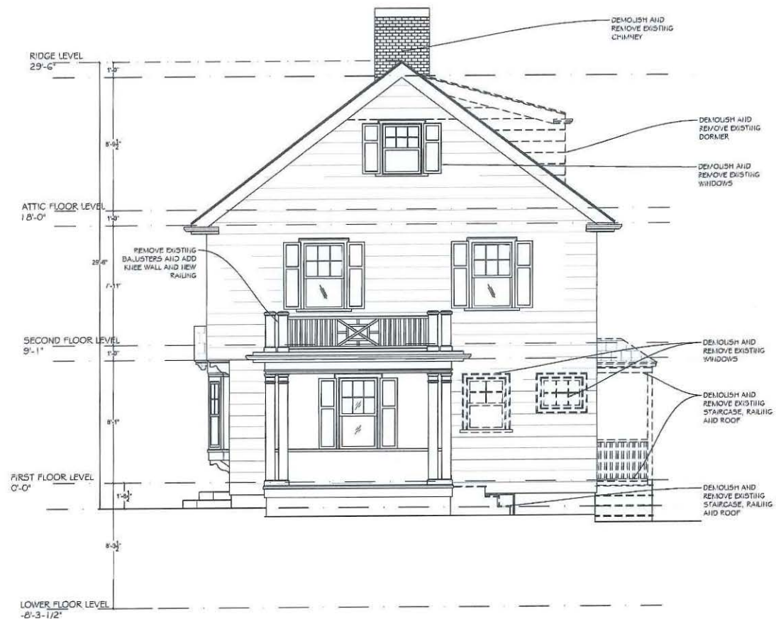
RIGHT ELEVATION - DEMOLITION SCALE: 1/4" = 1'-0"
