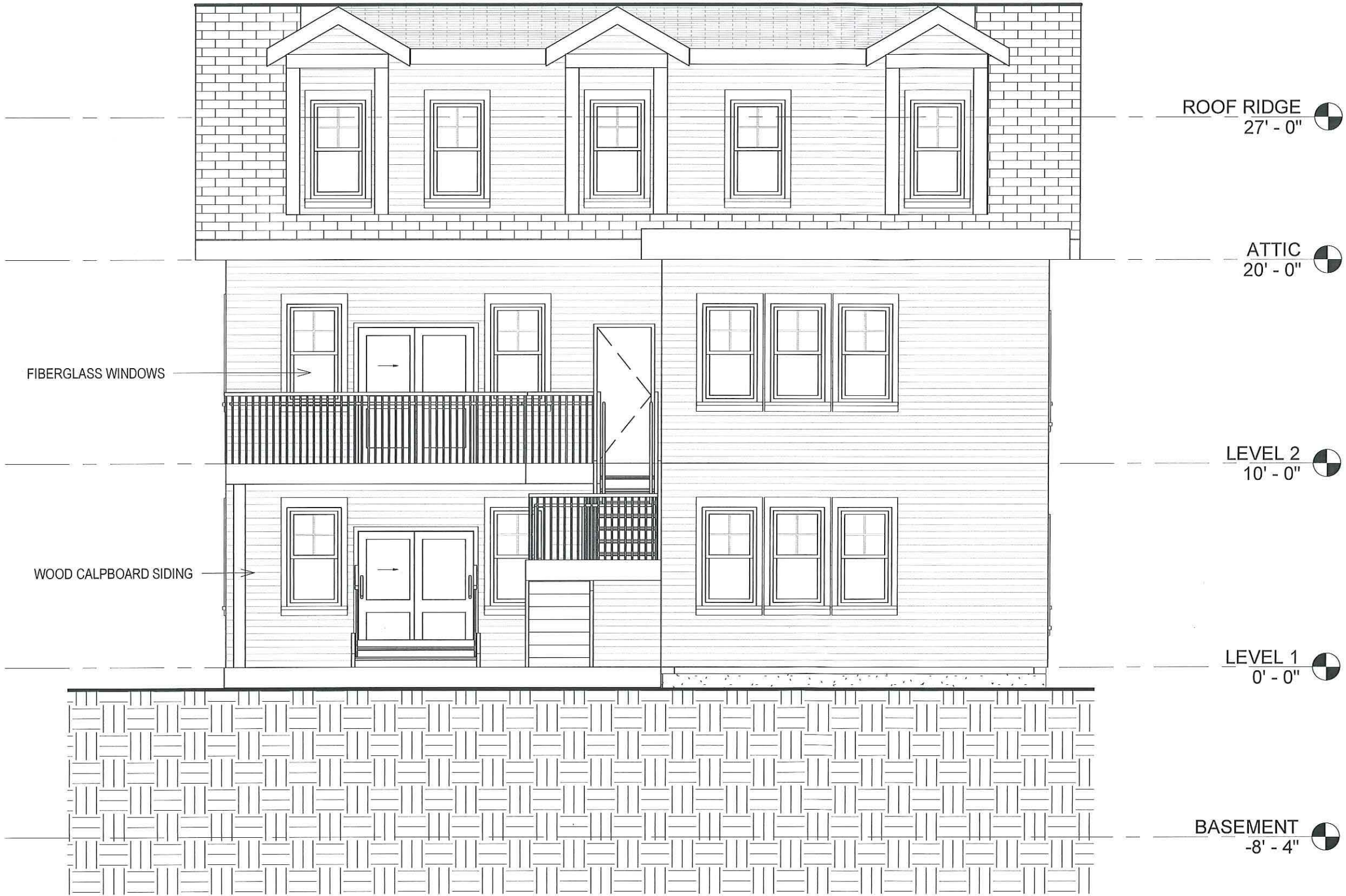
1 REAR ELEVATION - NEW A9a Scale: 3/16" = 1'-0"
