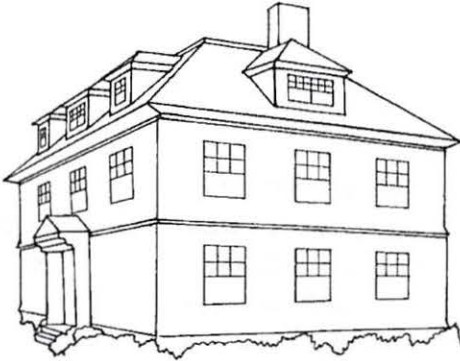
Figure 13: Gable dormers added in combinations, such as triplets, should be arranged symmetrically within the main roof so they are centered and spaced proportionally. The distance between each should be no less than one half (1/2) the width of the largest dormer.
