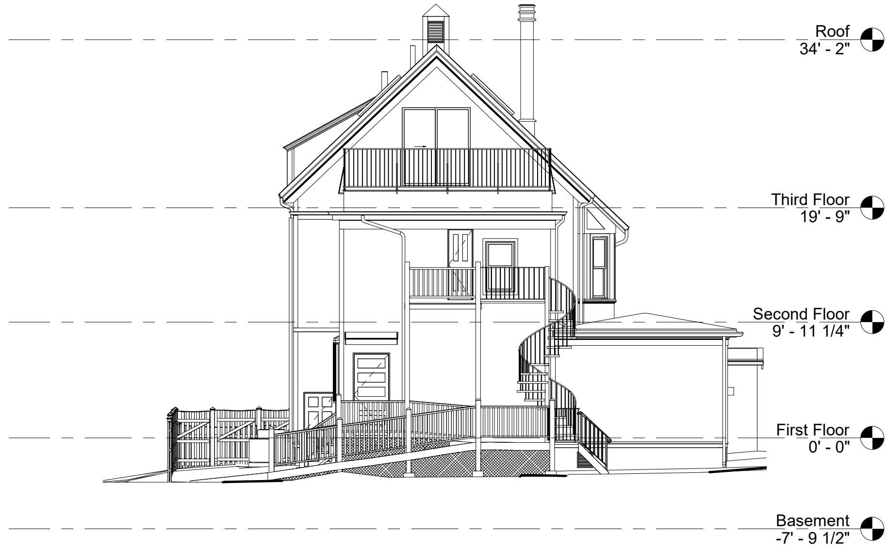
① North Elevation - Existing 1/8" = 1'-0"
