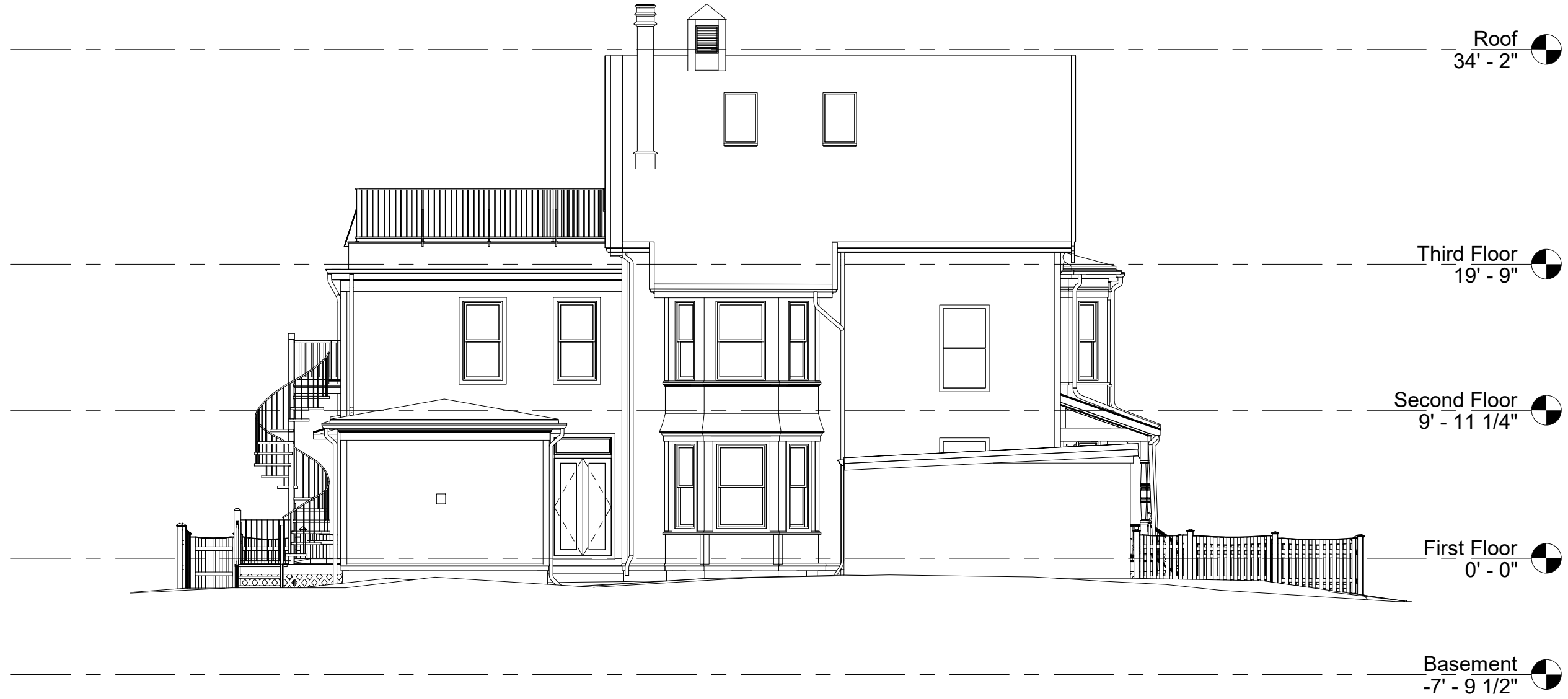
① West Elevation - Existing 1/8" = 1'-0"
