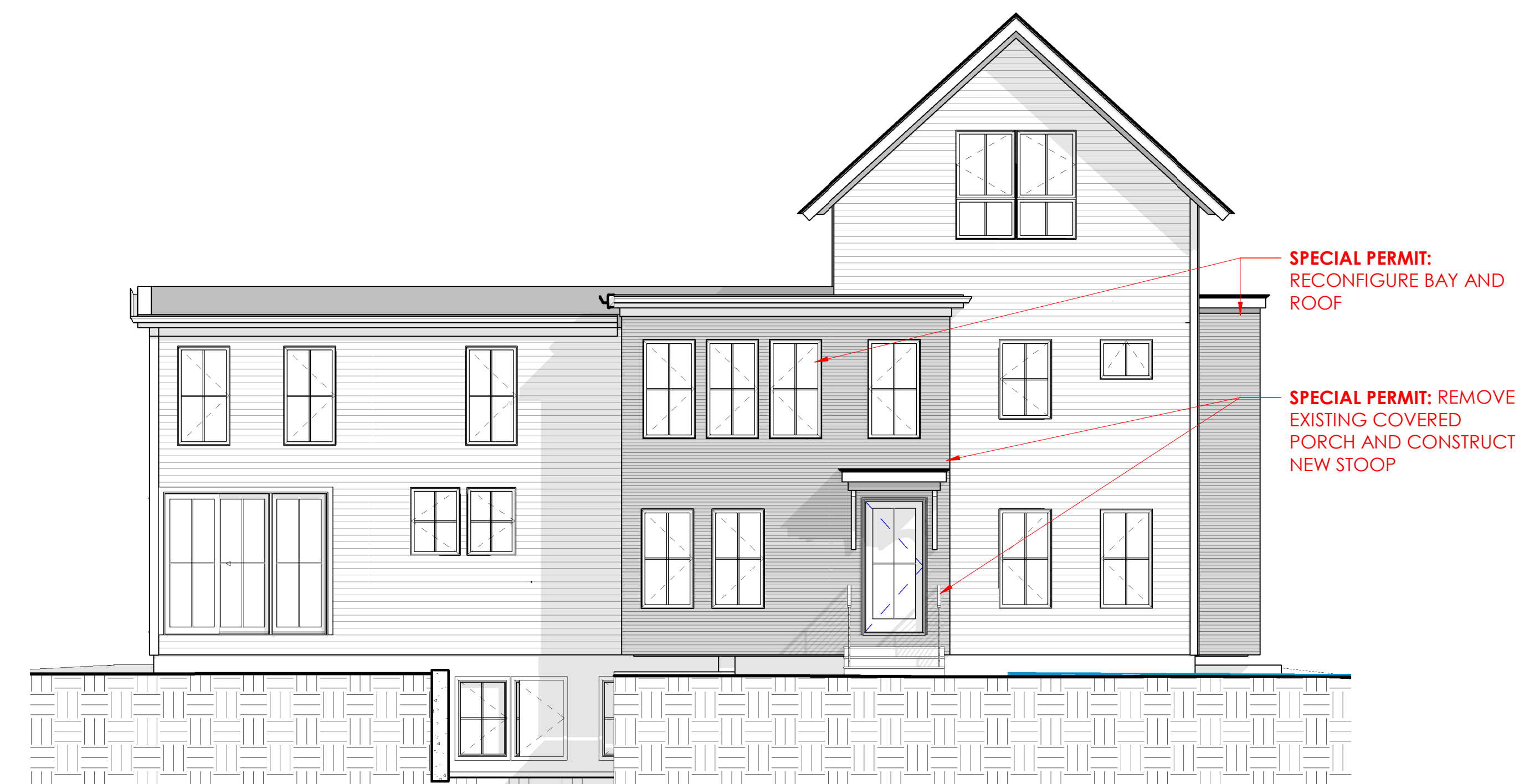
PROPOSED LEFT SIDE ELEVATION (BZA)
