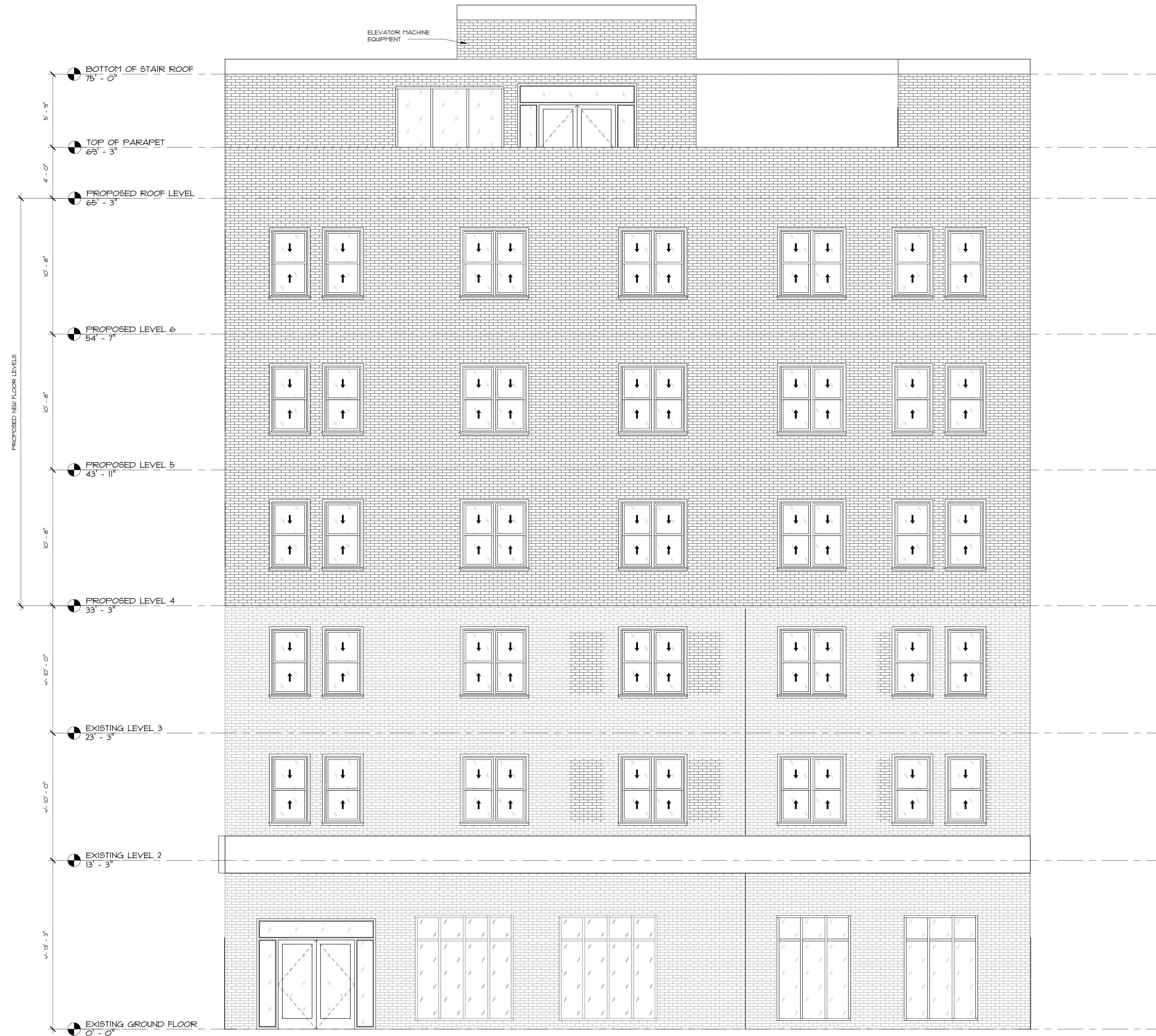
1 PROPOSED SOUTH EXTERIOR ELEVATION - CAMBRIDGE STREET SD3.1 1/4" = 1'-0"
