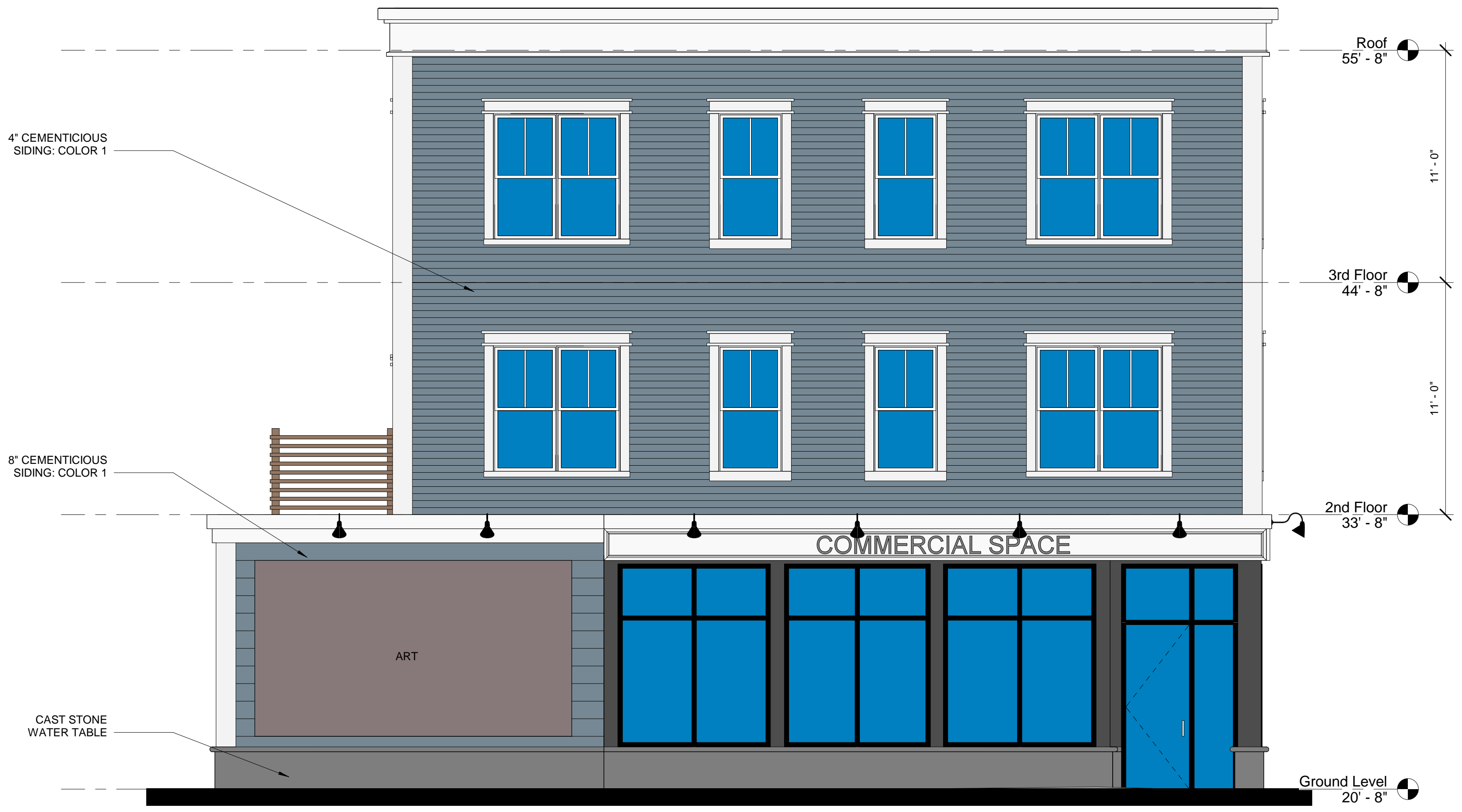
① Cambridge Street (South) Elevation 1/4" = 1'-0"
