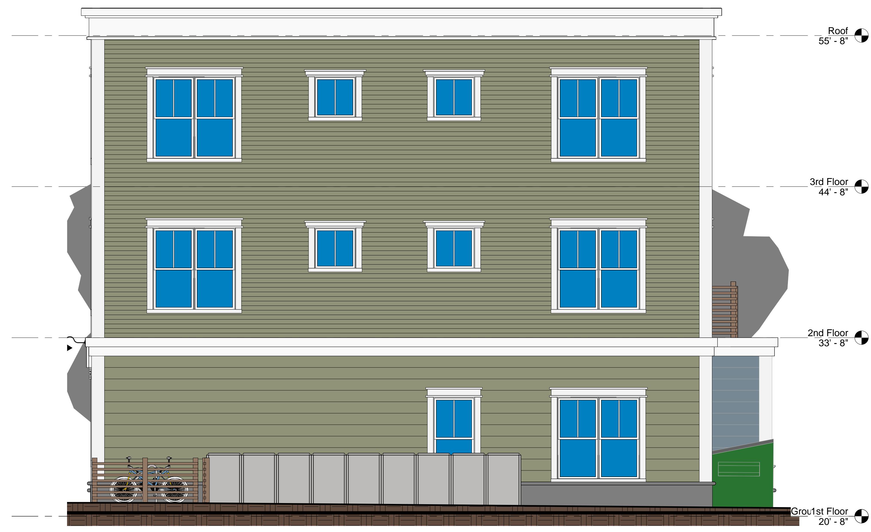
① Right Side (North) Elevation 1/4" = 1'-0"
