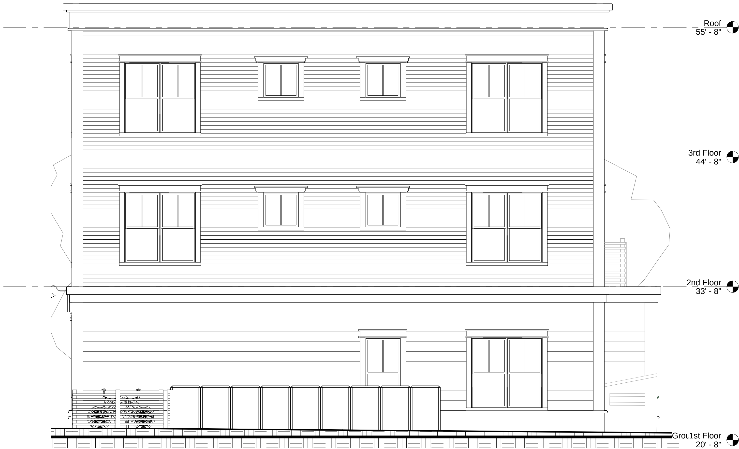
2 Right Side (North) Elevation 1/4" = 1'-0"
