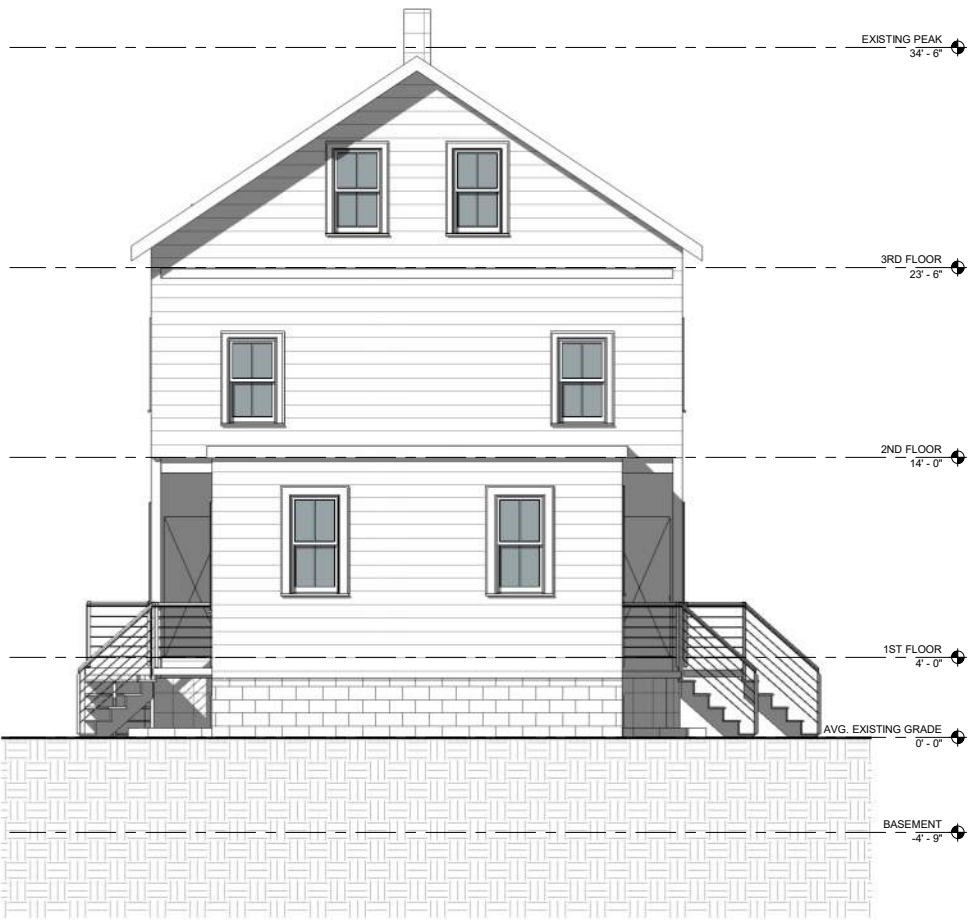
② EXISTING REAR ELEVATION 1/4" = 1'-0"
