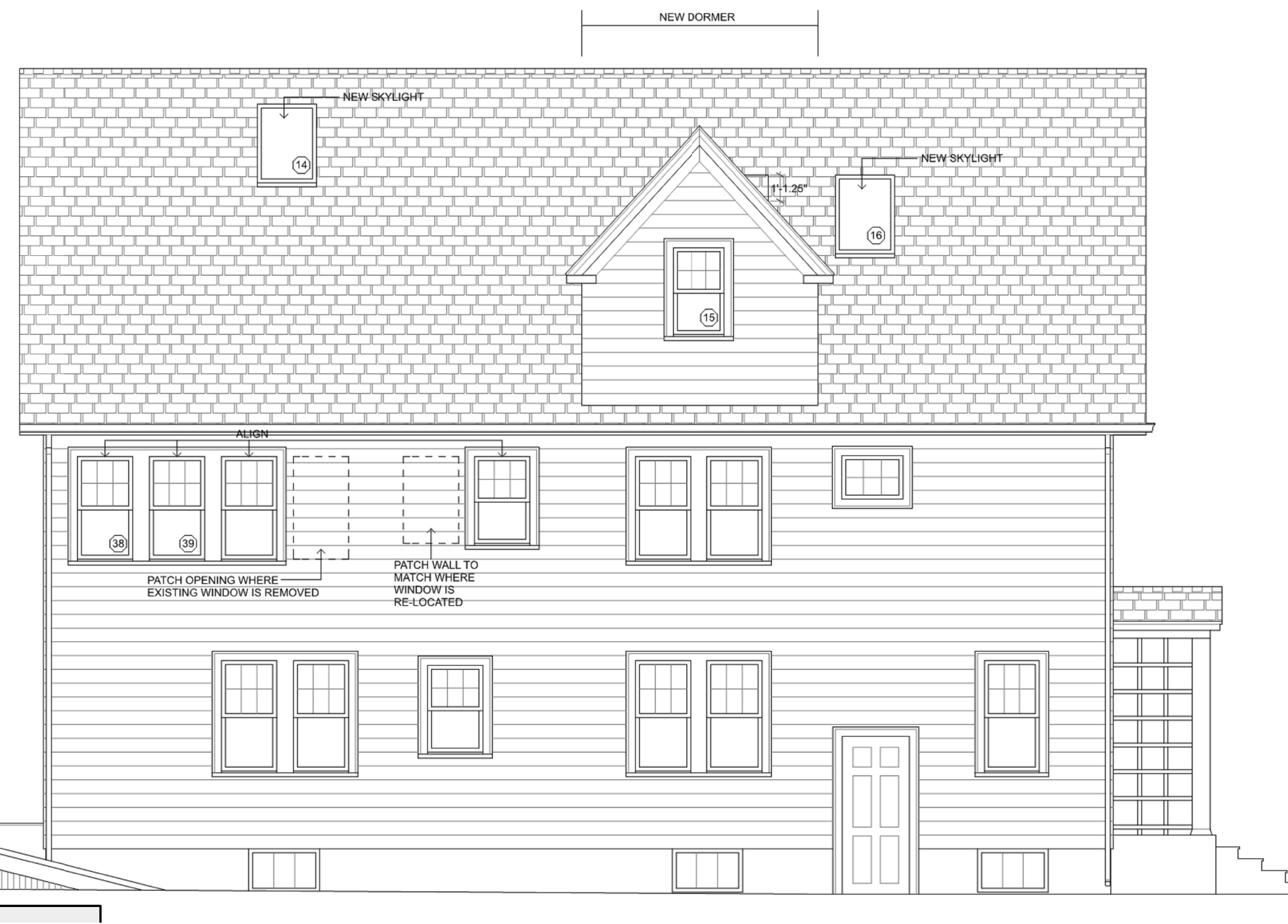
EXISTING WEST ELEVATION
