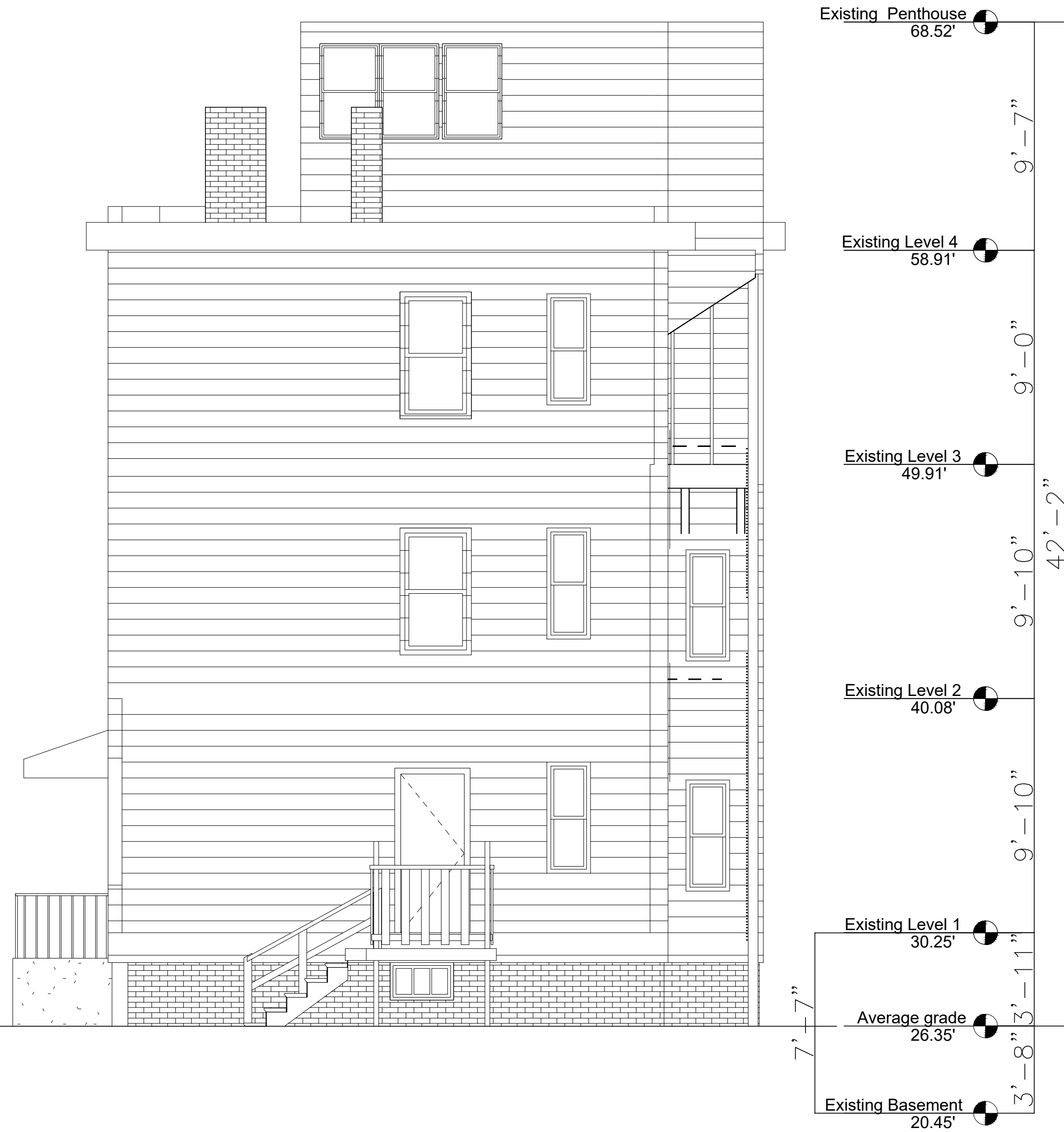
1 Existing Elevation: East Scale 1/4" = 1'-0"
