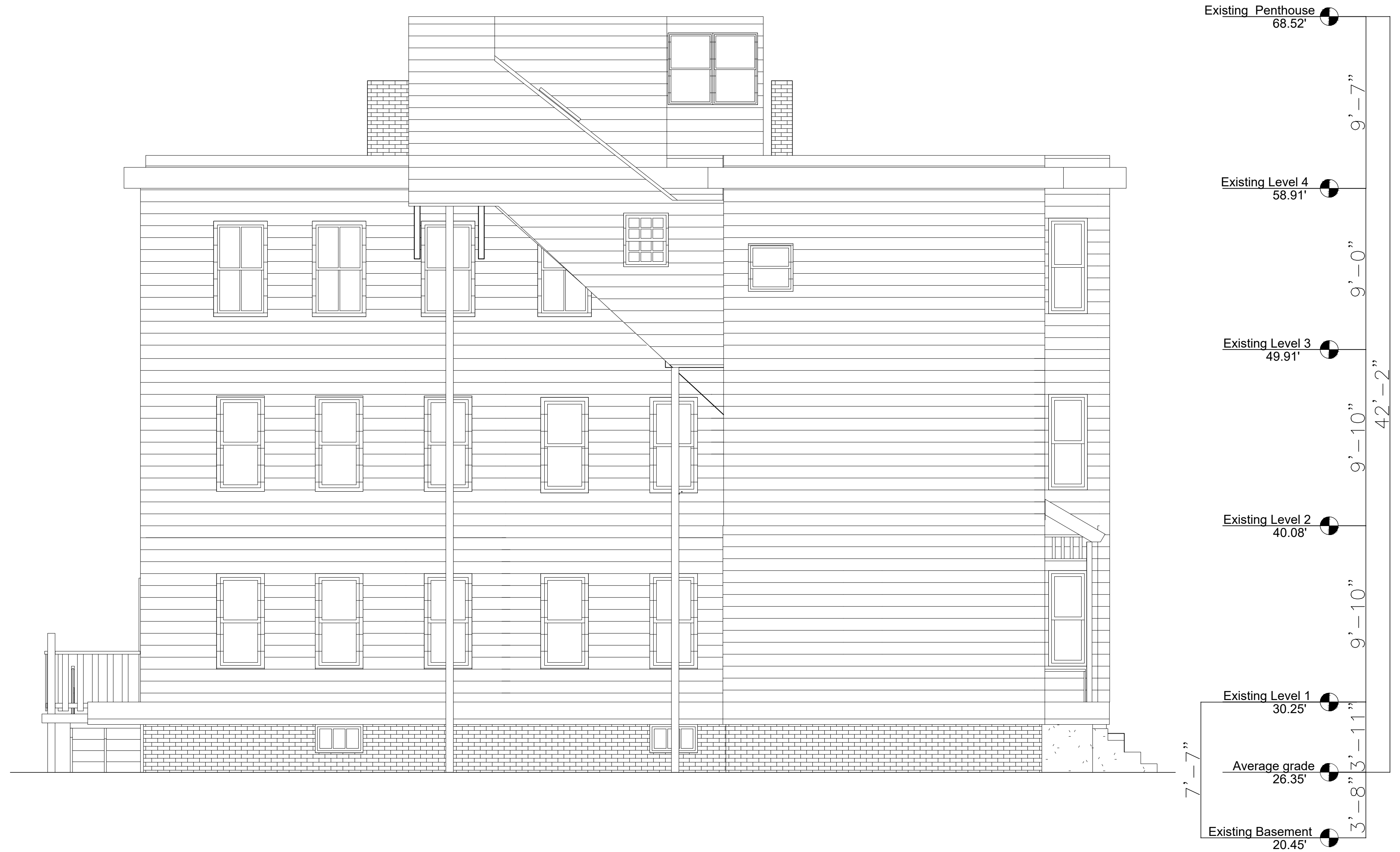
2 Existing Elevation: North Scale 1/4" = 1'-0"
