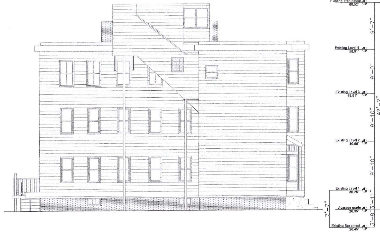
2 Existing Elevation: North Scale 1/4" = 1'-0"
