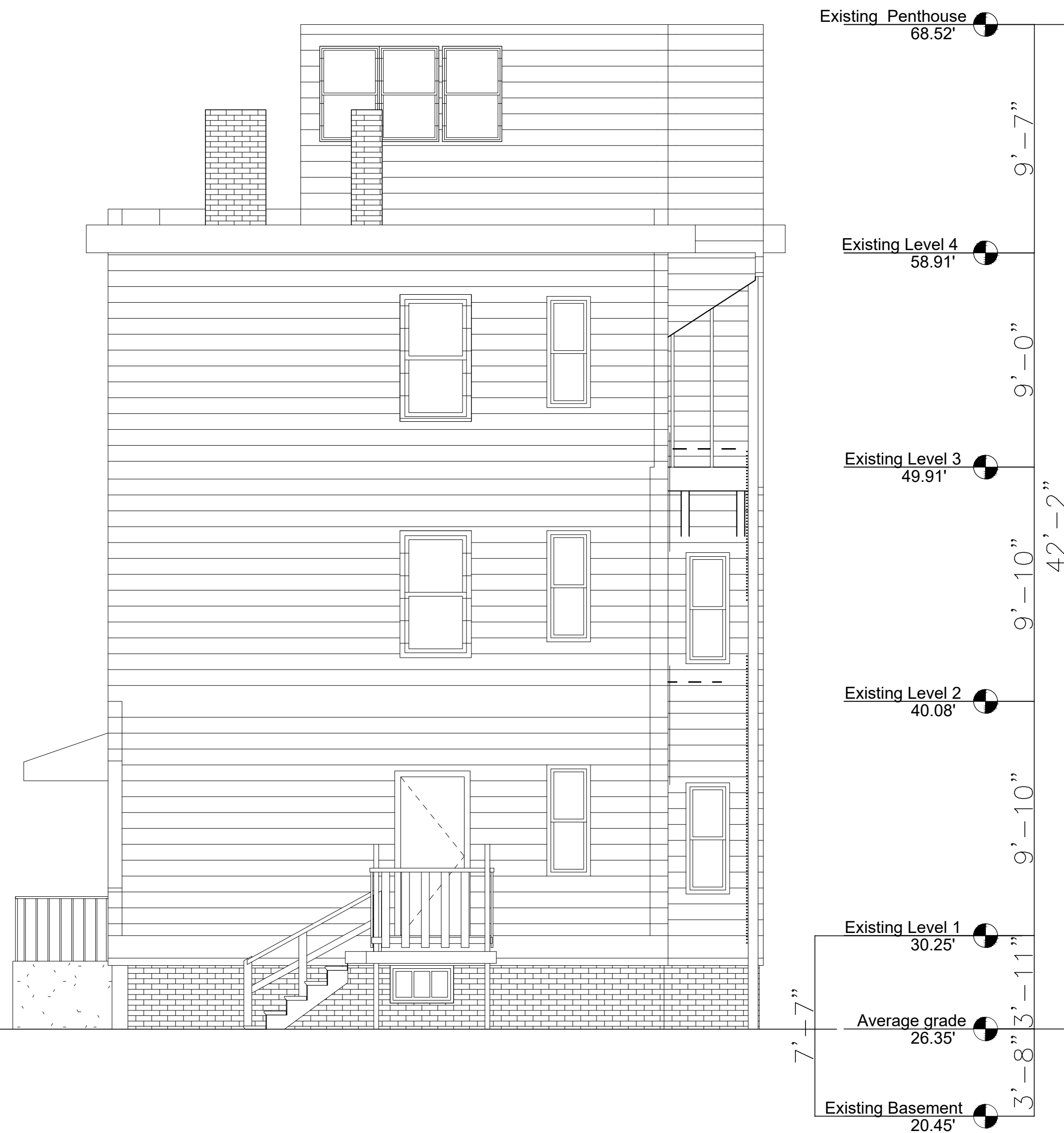
1 Existing Elevation: East Scale 1/4" = 1'-0"
