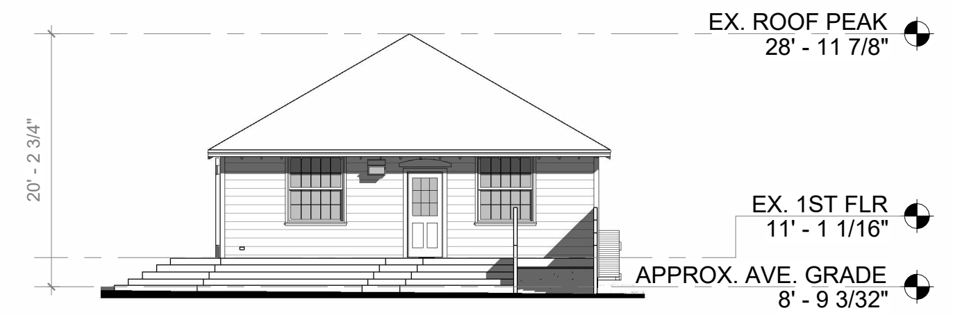
EXISTING SOUTH ELEVATION 3/32" = 1'-0"
