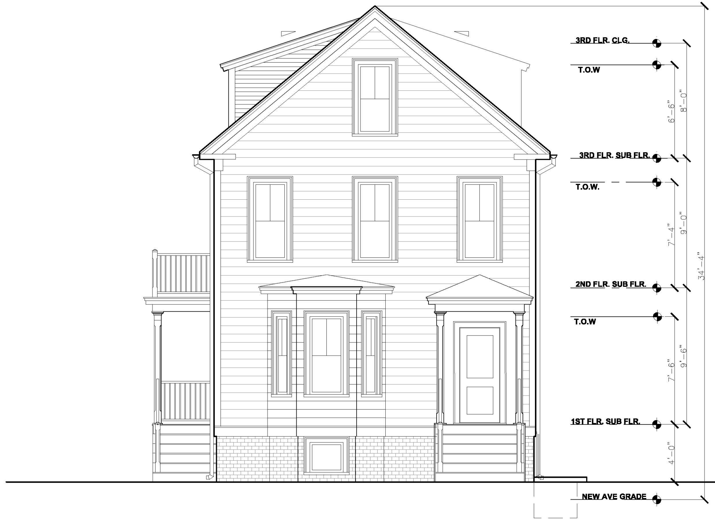
1 Elevation: East Scale 1/4" = 1'-0"
