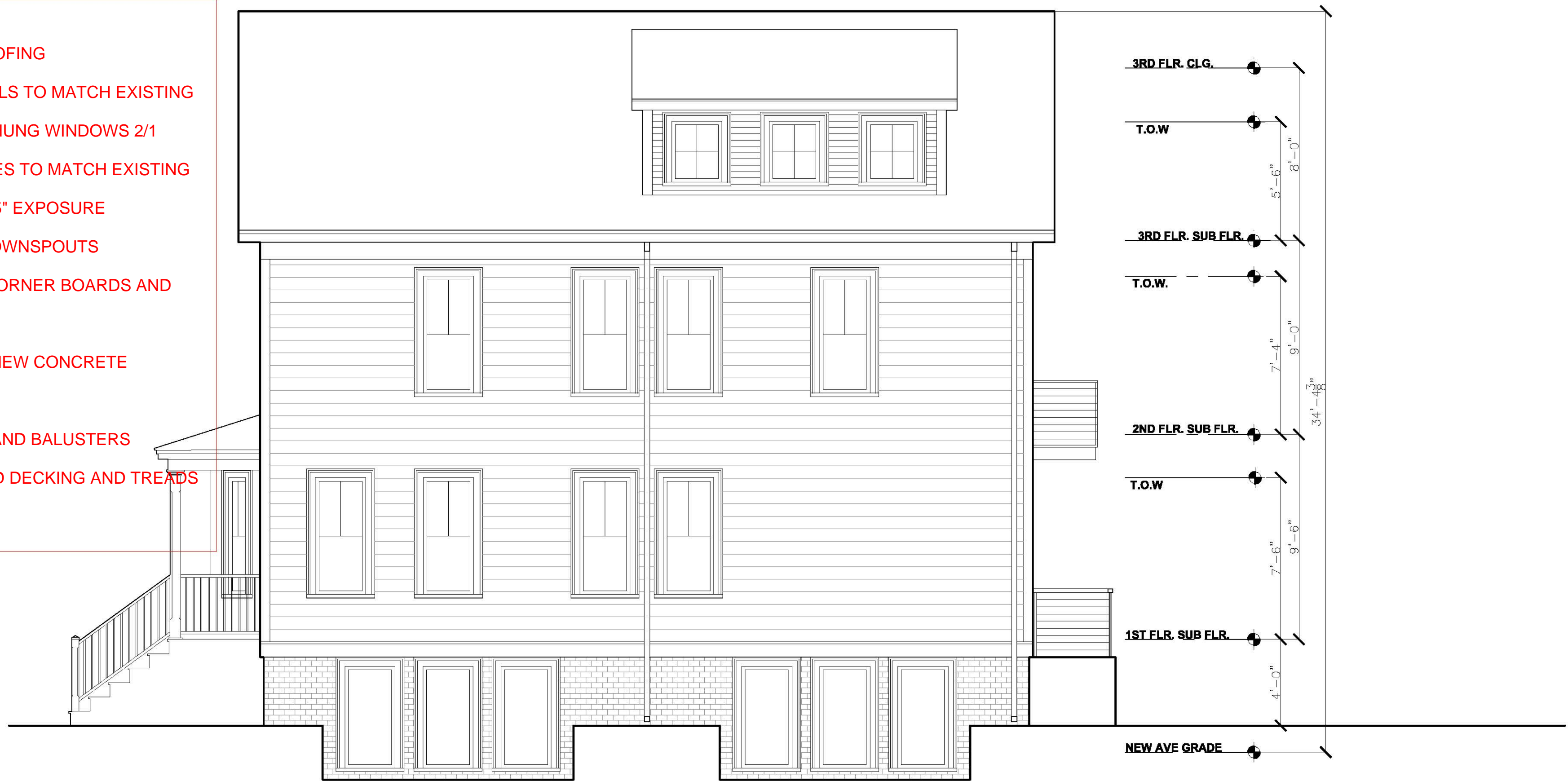
2 Elevation: South Scale 1/4" = 1'-0"
