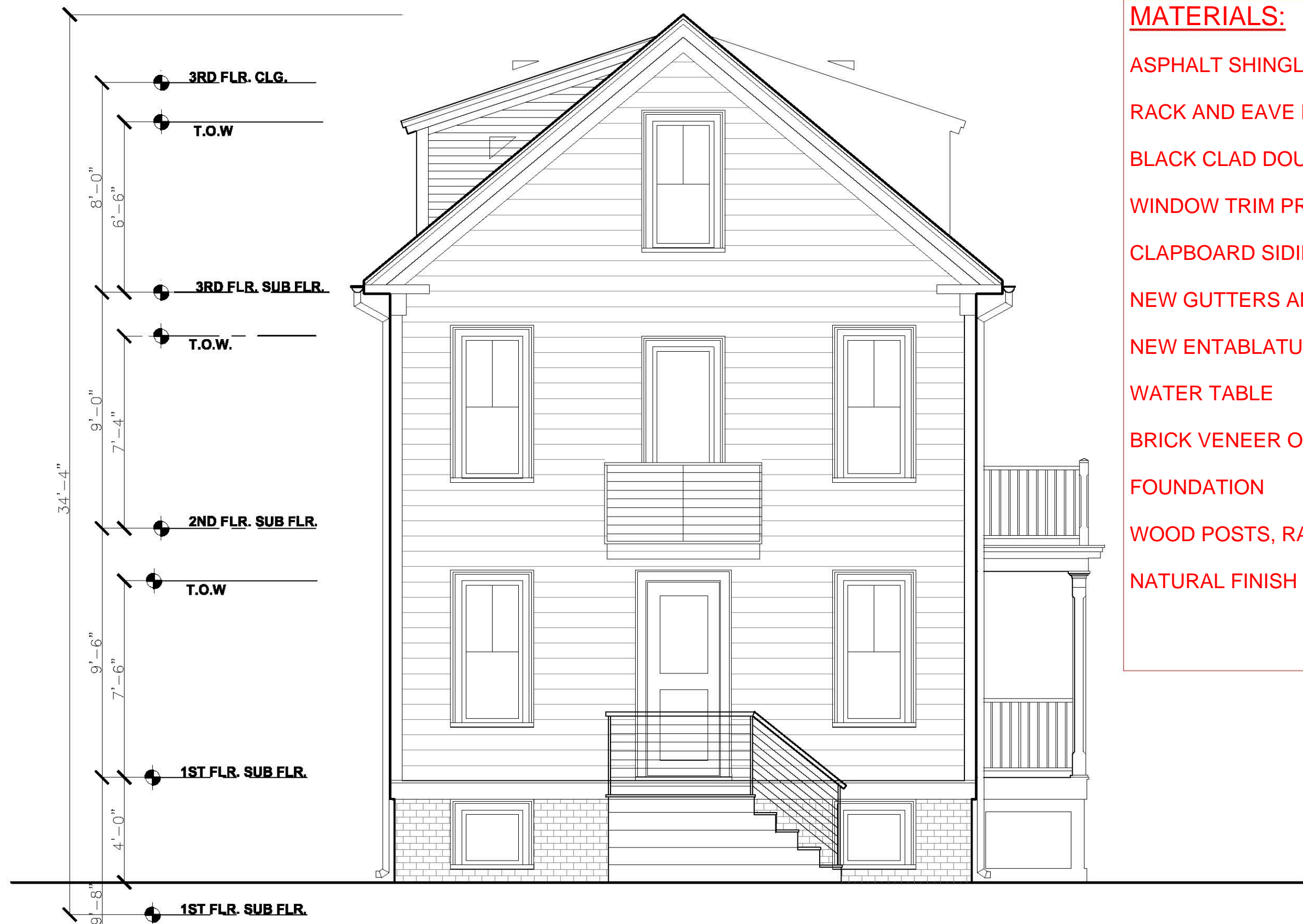
1 Elevation: East Scale 1/4" = 1'-0"
