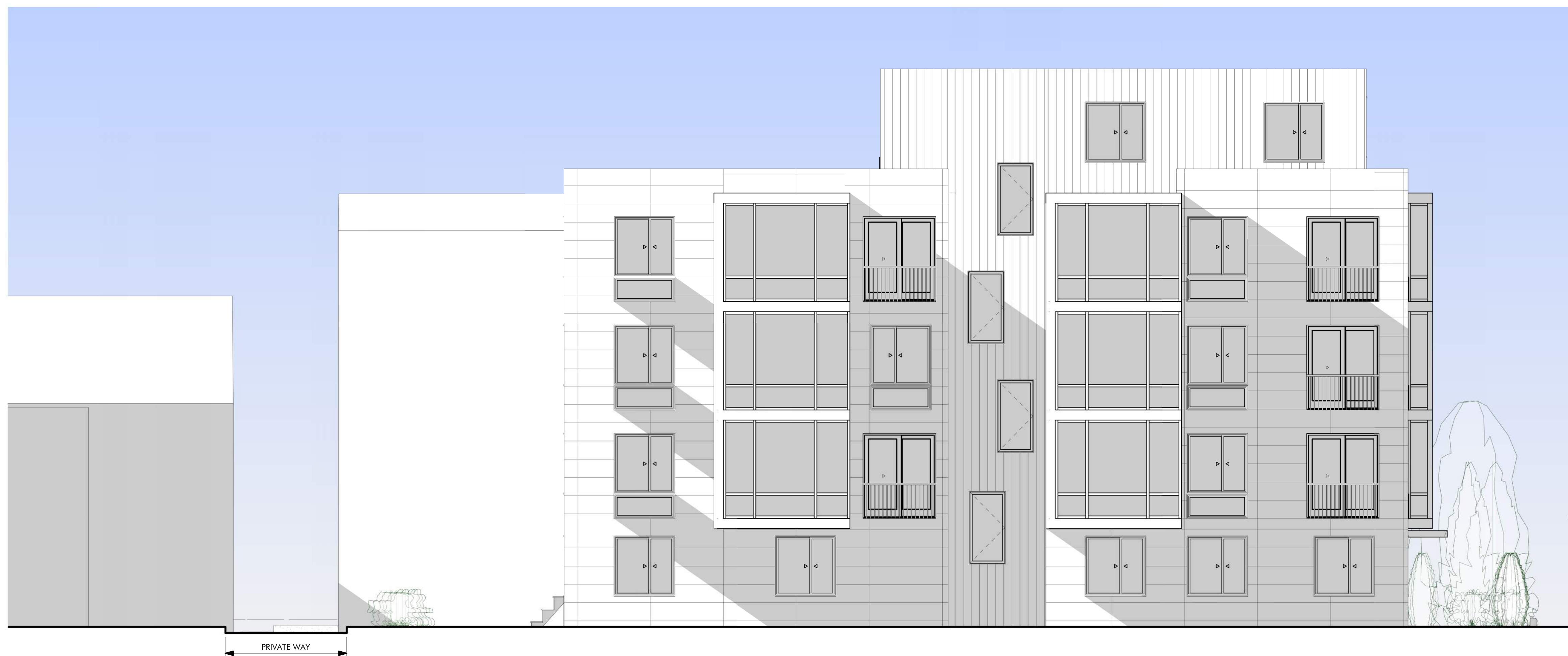
② PROPOSED SOUTH ELEVATION 3/16" = 1'-0"
