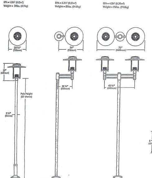
Single Arm Mount (IA) Dia-cast aluminum single luminoire
