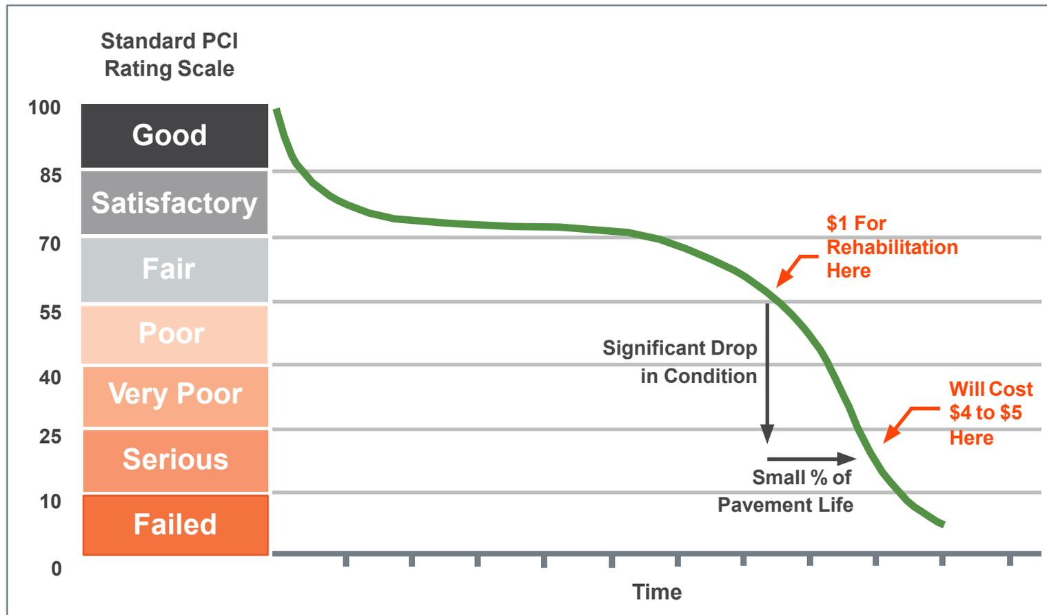
Based on the Pavement Condition Index (PCI), the City's average rating is 66.2. The average is holding steady year to year. A combination of capital construction and maintenance have resulted in a decrease of \$2.4 million in the backlog of repairs.
