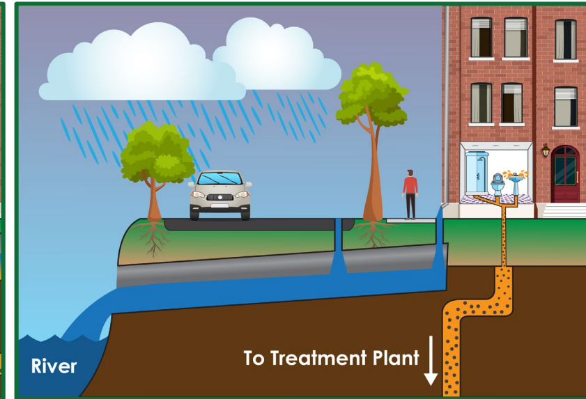
Separated System – All Rain
