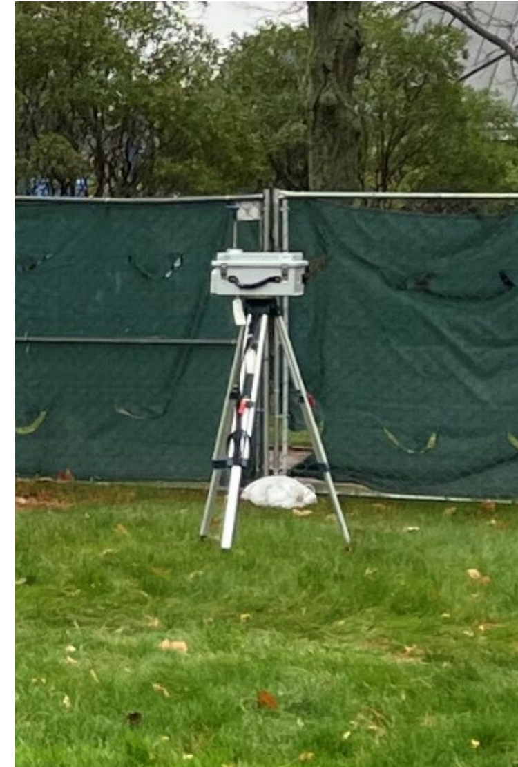
Example of dust monitoring equipment.
