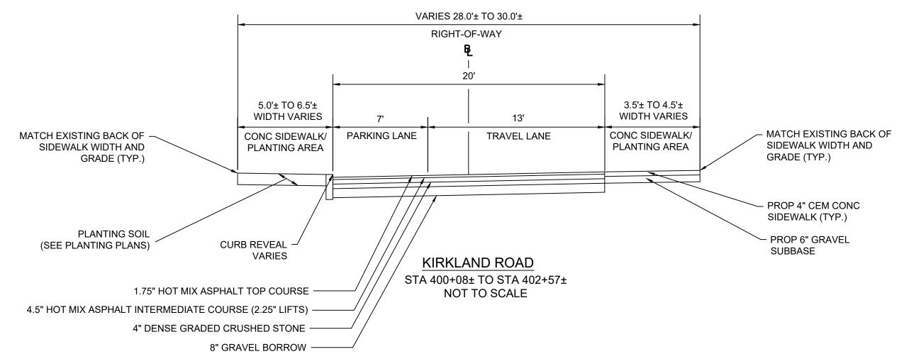
SURFACE: 1.75" HOT MIX ASPHALT SURFACE COURSE 12.5 (SSC-12.5) OVER 4.5" (2.25" LIFTS HOT MIX ASPHALT INTERMEDIATE COURSE 19.0
