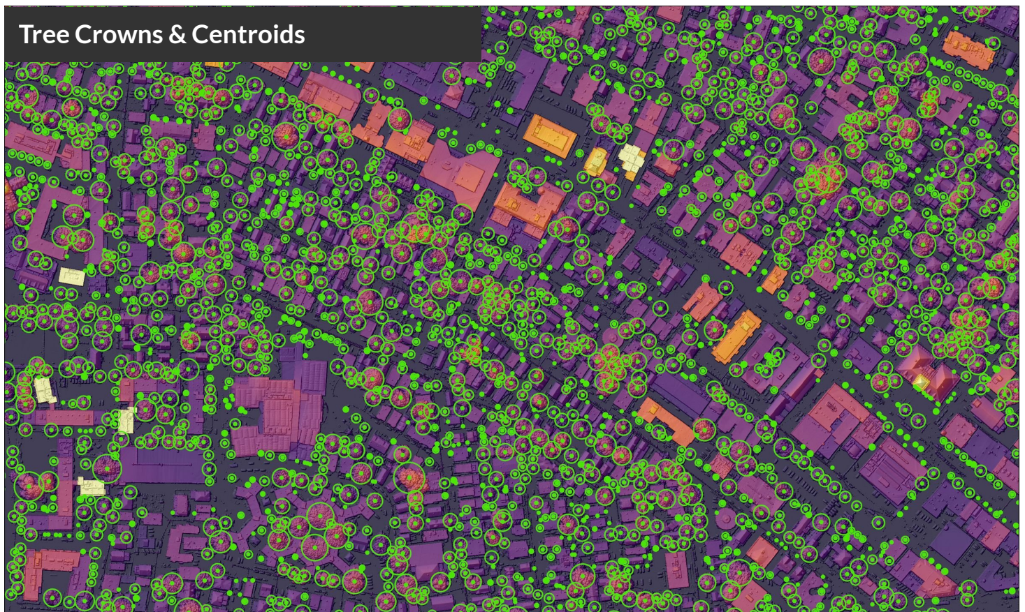
Figure 4. Tree centroids (dots) and tree crowns (circles) mapped from the 2024 LiDAR. Tree mapping from LiDAR involves finding relative high points for each tree, then tracing down until a height inflection point is reached, marking the edge of the crown. This approach to individual tree mapping is most accurate where there is a clear differentiation in tree crowns and is less accurate in forested stands where crowns may overlap.
