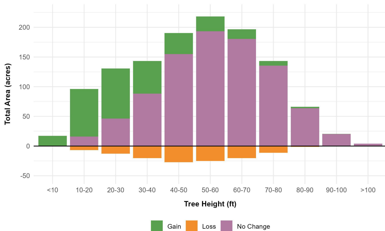
Figure 22. The tree canopy was segmented into polygons approximating individual trees. Each of these polygons was then attributed with the height from both the 2019 and 2024 LiDAR data. The height from the 2019 LiDAR was used to understand loss (orange), whereas the height from the 2024 LiDAR was used to understand the gains (green) and no change (purple).
