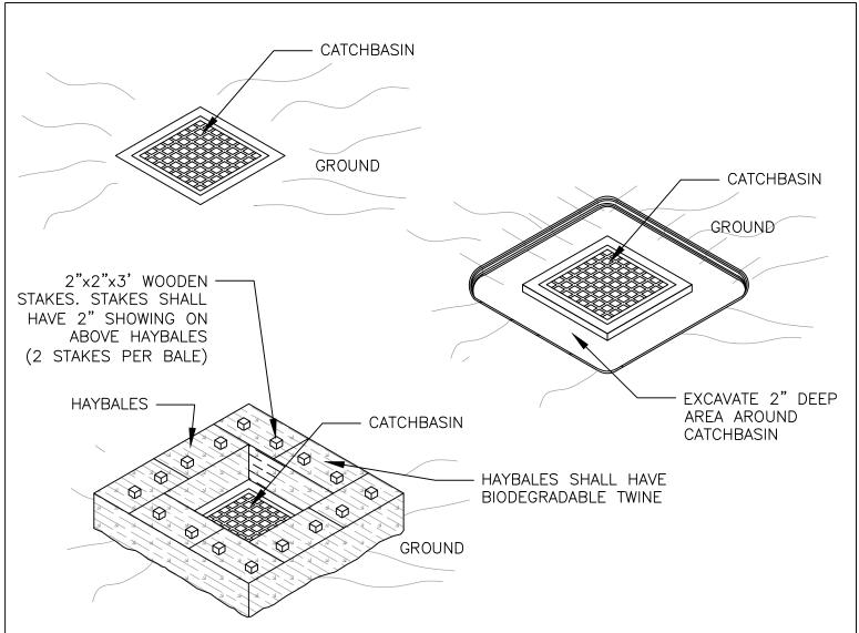
INSPECTION SCHEDULE SHALL COMPLY WITH THE 2008 EPA CONSTRUCTION GENERAL PERMIT THIS METHOD OF INLET PROTECTION IS APPLICABLE WHERE THE INLET DRAINS A RELATIVELY FLAT AREA (SLOPE NO GREATER THAN 5%). WHERE THE INLET ACCEPTS SHEET OR OVERLAND FLOWS (NOT GREATER THAN 1 CFS). THIS METHOD SHOULD NOT APPLY TO AN INLET ACCEPTING CONCENTRATED FLOW.
