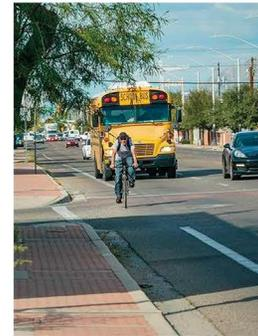
Like River Street, the image to the left shows a narrow bike lane that leaves the biker exposed to on-coming traffic. This type of facility represents a BLC 3 based on traffic volume, vehicle speeds and the number of travel lanes.
