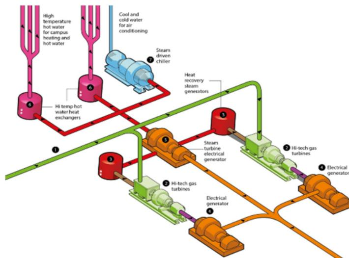
Figure 10. Gas-fired cogeneration plant [Source: New York University]
