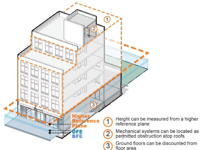
Figure 9. New Dry Floodproofed Mixed-Use Building.
