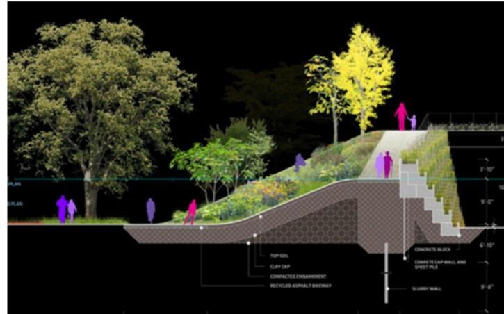
Figure 1. Raised berm for flood protection [Source: Rebuild By Design]
