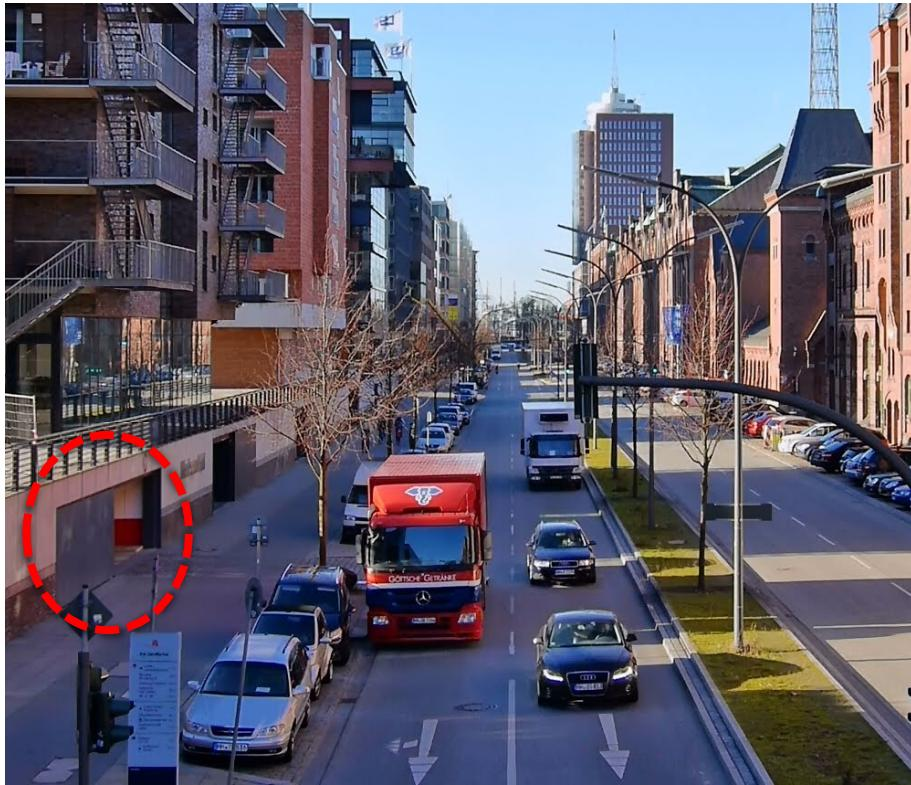
In HafenCity, Hamburg, Germany, building facades are designed as continuous flood wall. [Source: <http://www.hafencity.com/en/concepts/flood-secure-bases-instead-of-dikes-safe-from-high-water-in-hafencity.html>]
