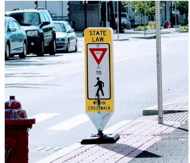
In-street pedestrian crosswalk signs
