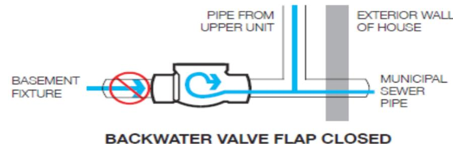
During a rainfall or sewer backup event, the backwater valve closes to block sanitary sewage from entering your basement fixtures. Please be aware that closed valves also prevent basement wastewater from exiting into municipal sewer pipes.
