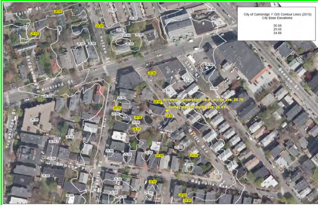
Figure 13: High water elevation from July 10, 2010 flood on Myrtle Ave (Source: City of Cambridge)<sup>16</sup>
