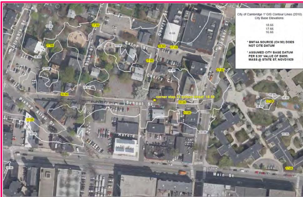
**Figure 8: High water elevation from July 10, 2010 flood on School St** (Source: City of Cambridge)<sup>11</sup>
