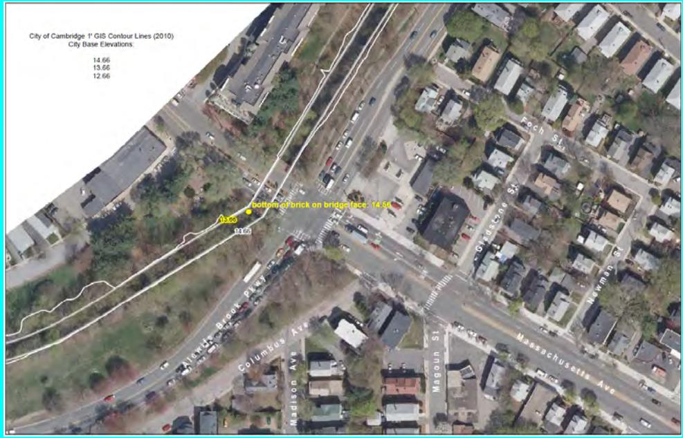
Figure 3: High water elevation from July 10, 2010 flood at Massachusetts Ave and Alewife Brook Pkwy (Source: City of Cambridge)<sup>6</sup>
