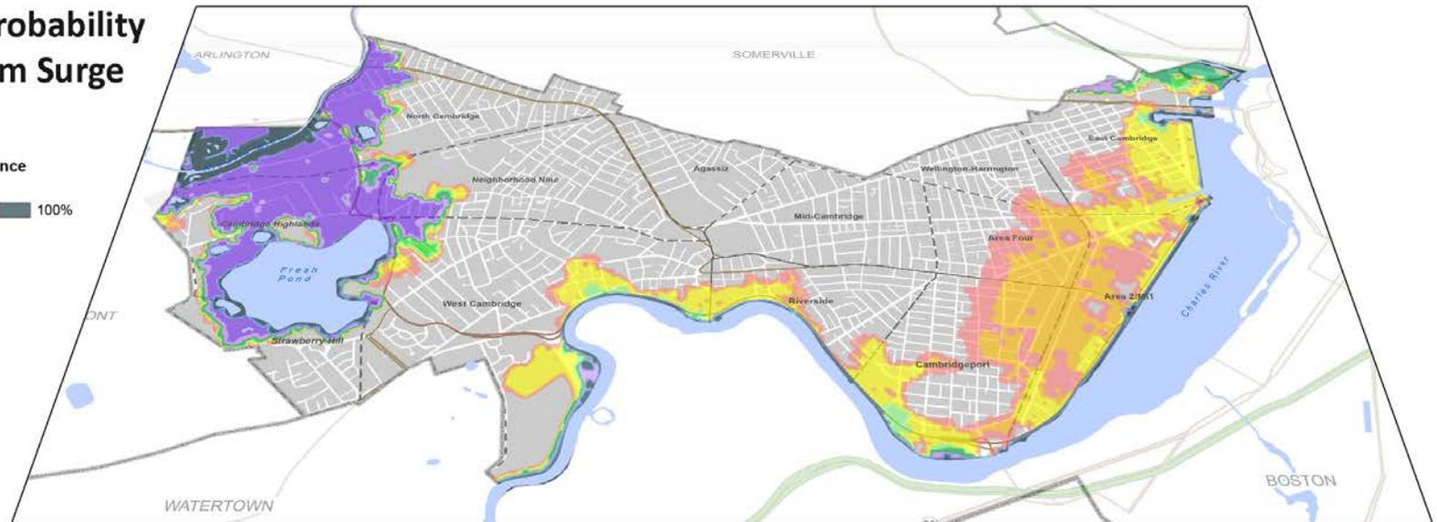
Fig. 9 Top map: **2070 Depth of Flooding from SLR and Storm Surge at 1% Probability** Bottom map: **2070 Percent Probability of Sea Level Rise and Storm Surge Flooding** (Source: Kleinfelder, February 2017, based on WHG MassDOT Boston Harbor Flood Risk Model)
