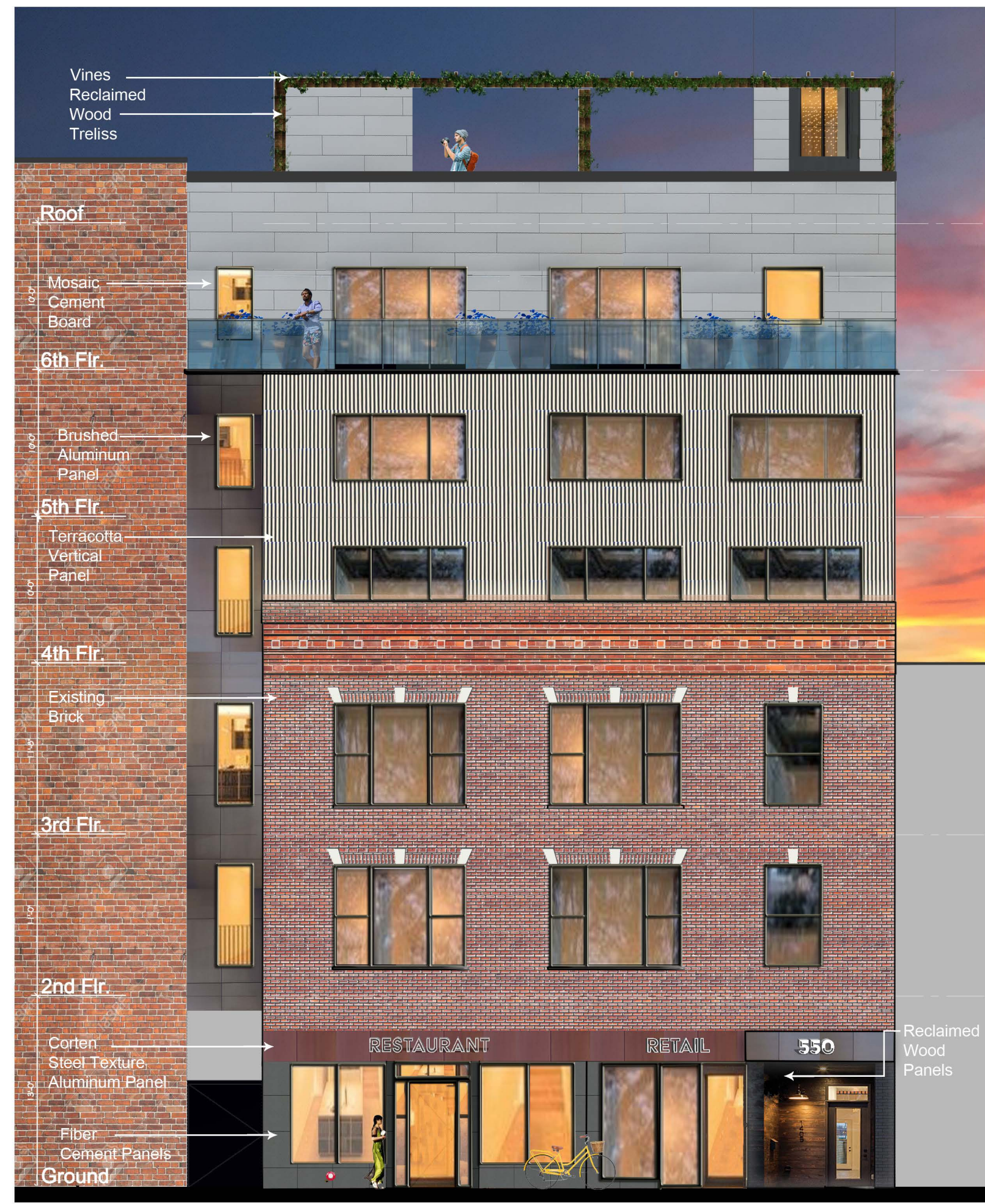
1 NORTHEAST ELEVATION Scale 1/8" = 1'-0"
