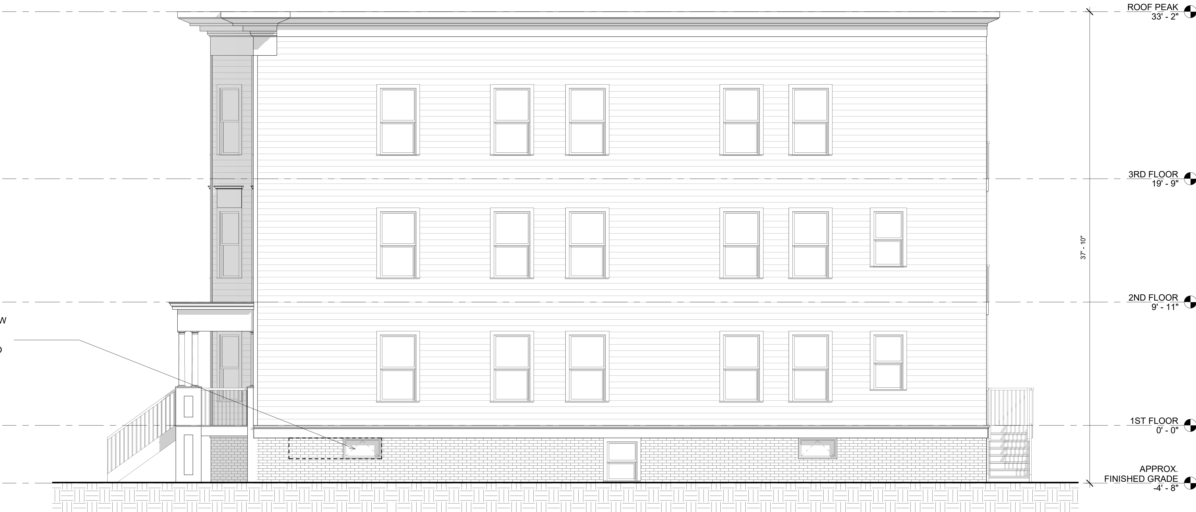
① EXISTING EAST ELEVATION 1/4" = 1'-0"
