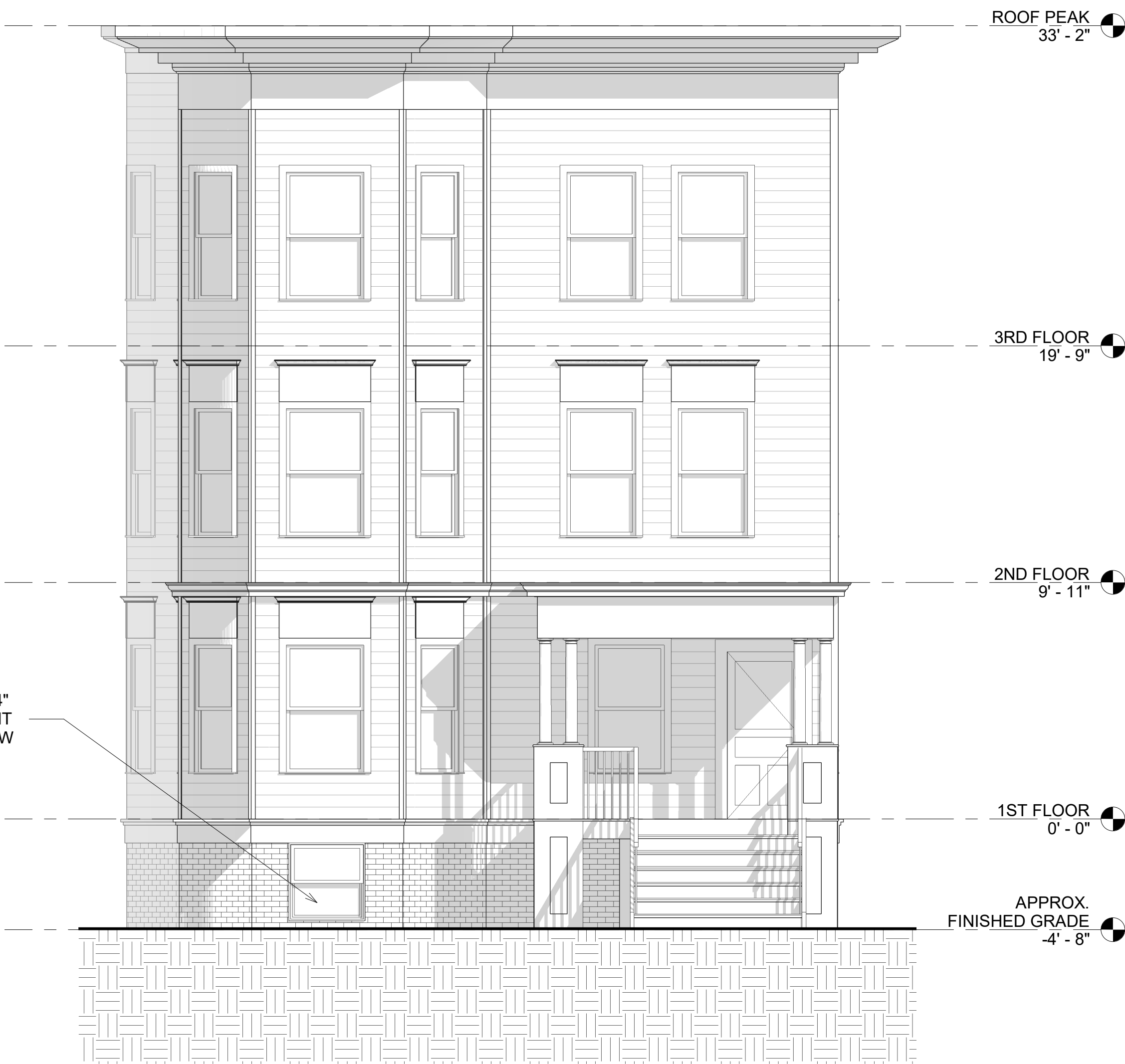
① PROPOSED SOUTH ELEVATION 1/4" = 1'-0"
