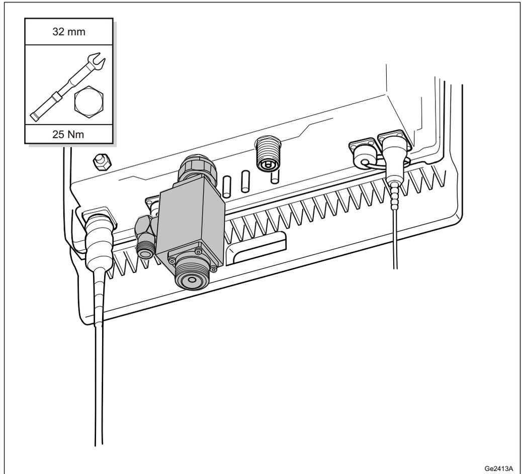
Figure 14 RF Monitoring Interface Connection
