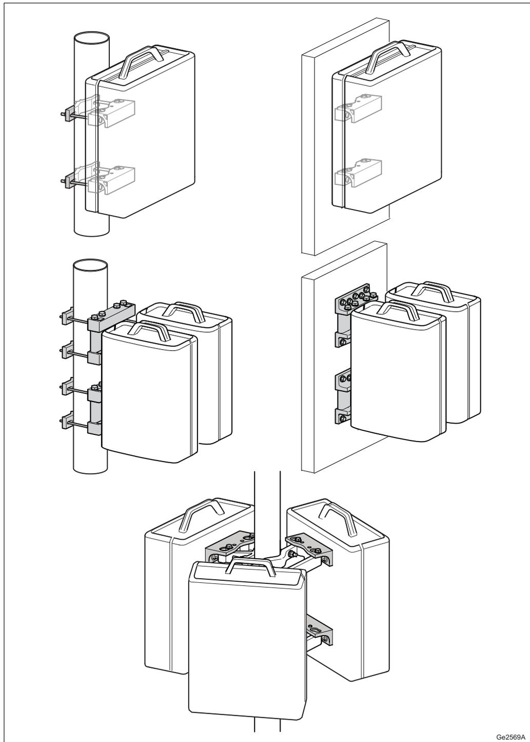
*Figure 4 Installation Alternatives*
