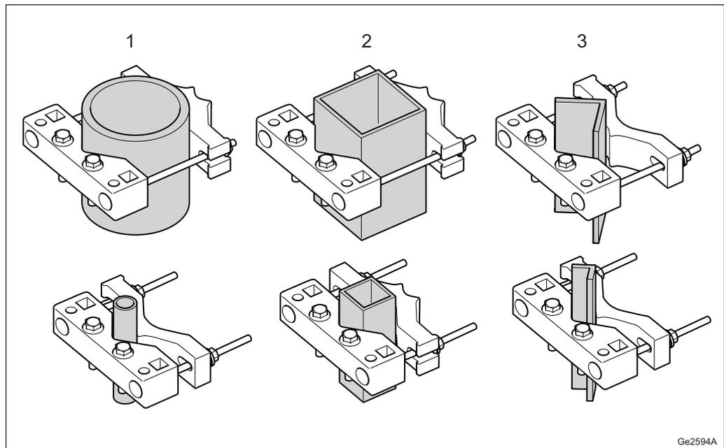
Figure 5 Alternative Pole or Mast Cross Sections
