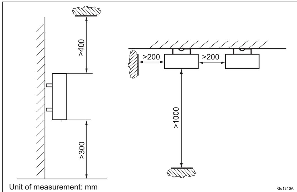
Figure 4 RRUS Wall Installation Requirements
