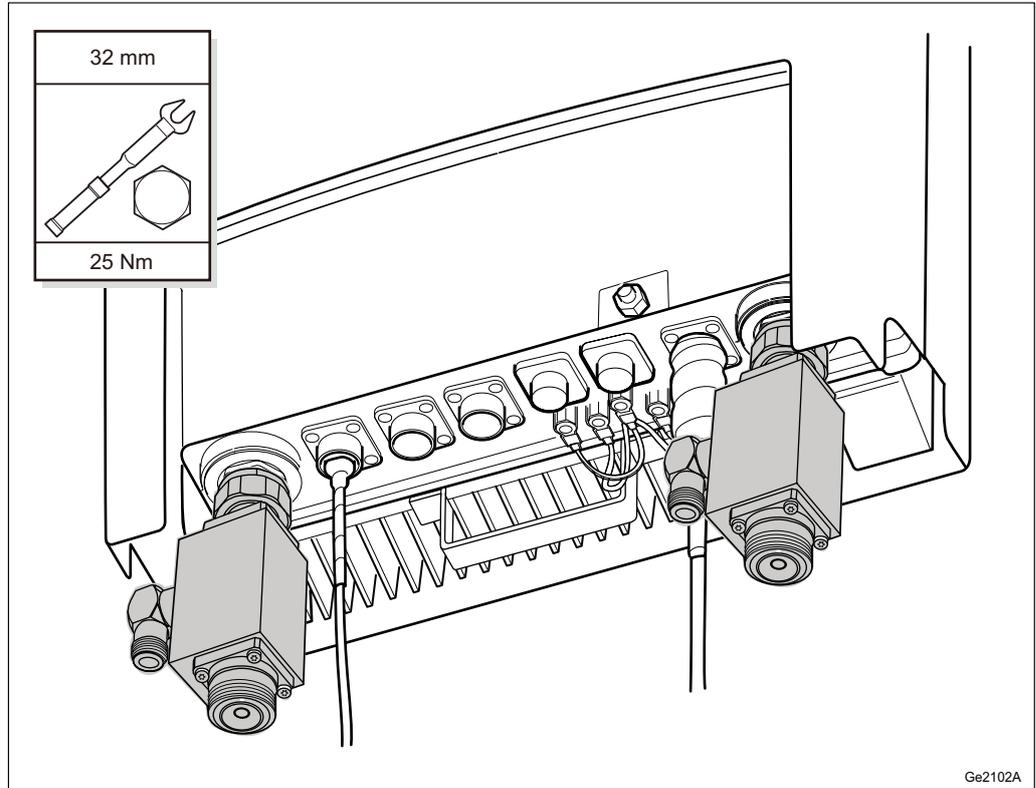
Figure 13 RF Monitoring Interface Connection
