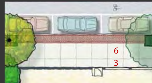
Concrete scoring with a 2:1 ratio
