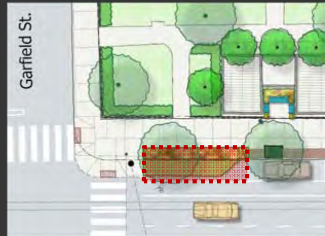
Possible rain garden on curb extension at Garfield St.
