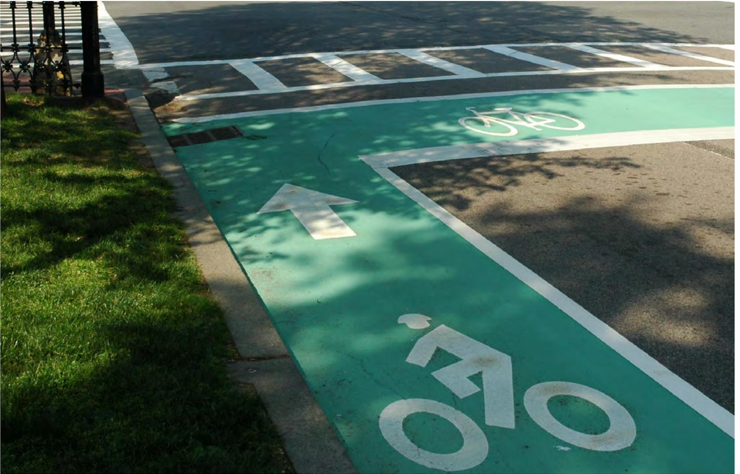
A bike box is a designated area at the head of a traffic lane at a signalized intersection that provides bicyclists with a safe and visible way to get ahead of queuing traffic during the red signal phase. They increase visibility of bicyclists and reduce signal delay for bicyclists. Bike boxes that extend across an entire intersection can also facilitate bicyclist left turn positioning during red lights.
