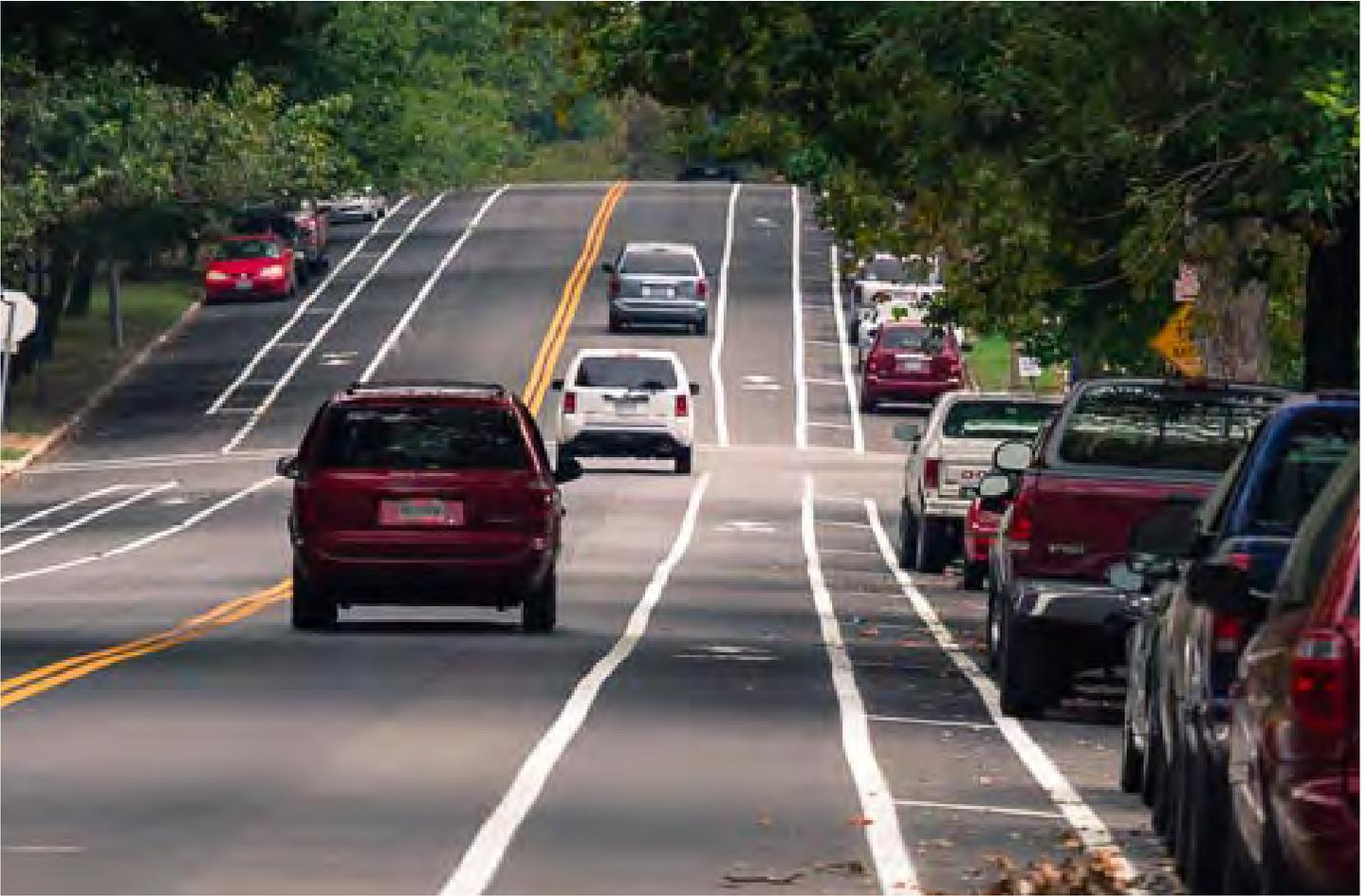
Buffered bike lanes are conventional bike lanes with a designated buffer space separating the bicycle lane from the parking lane. Benefits include reduced risk of “dooring” and greater space for cyclists to maneuver. Potential disadvantage is that motorists and delivery vehicles are more likely to illegally park in the lane.
