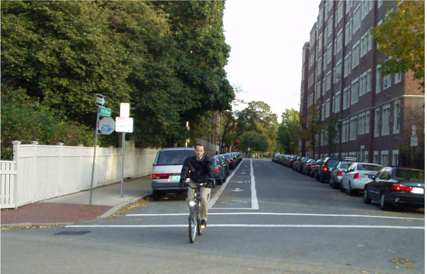
Contraflow bicycle lanes are bicycle lanes designed to allow bicyclists to ride in the opposite direction of motor vehicle traffic. They convert a one-way traffic instreet into a two-way street: one direction for motor vehicles and bikes, and the other for bikes only. One advantage is that they can provide more direct connections for cyclists.
