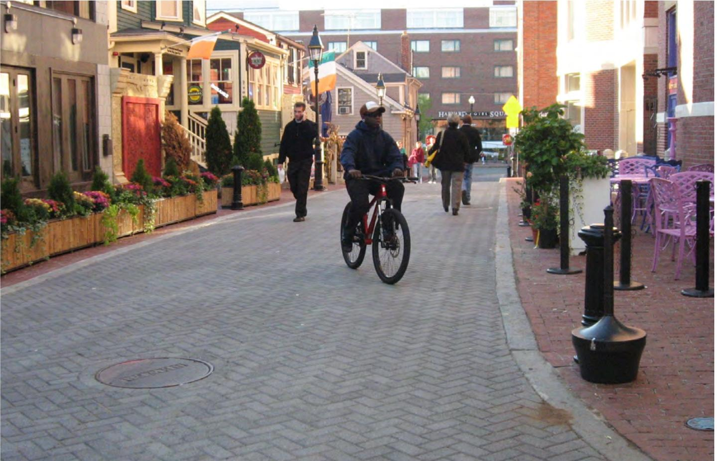
A shared street in this meaning is one where there is no curbed delineation between the roadway and the sidewalk and all users share the space. Vehicle volumes are either low or discouraged. The concept is also known as a “woonerf” (a Dutch term loosely translated into “living street”).
