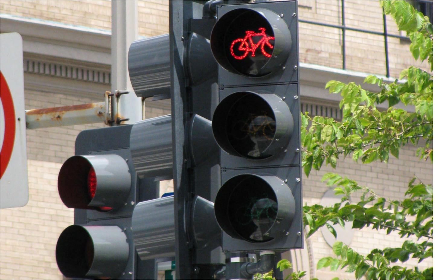
Bicycle signals and beacons facilitate bicyclist crossings of roadways. Bicycle signals make crossing intersections safer for bicyclists by clarifying when to enter an intersection and by restricting conflicting vehicle movements.
