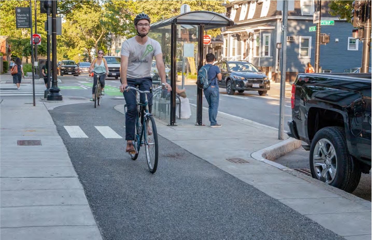
A floating bus stop creates a dedicated passenger platform between the motor vehicle lane and the bike lane. Bus passengers must cross the separated bike lane when entering and exiting the platform.
