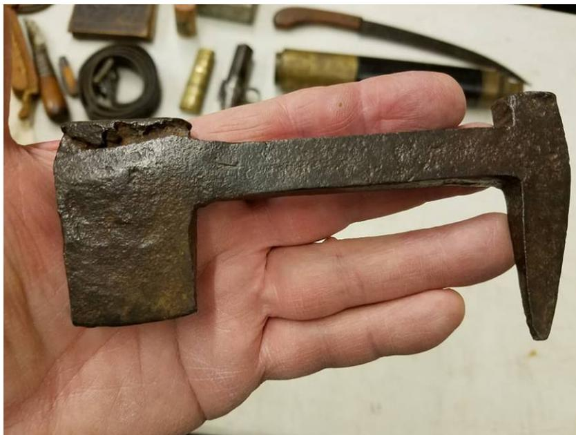
He couldn't help but notice the resemblance that if you modified these tools by removing the blade and attaching a chain and loop, it looks very much like the ladder dogs used today.
