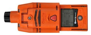
Each Ladder company now has a five sensor meter: Lower Explosive Limits (LEL), Oxygen (O2), Hydrogen Sulfide (H2S), Carbon Monoxide (CO), and **Nitrogen Dioxide (NO2)**.
