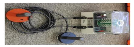
The MBTA Third Rail Tester is an audible and lighted warning device that alerts firefighters if the third rail is energized or de-energized. The third rail carries 600 volts of direct electrical current. The following instructions should be followed when using the third rail tester.
