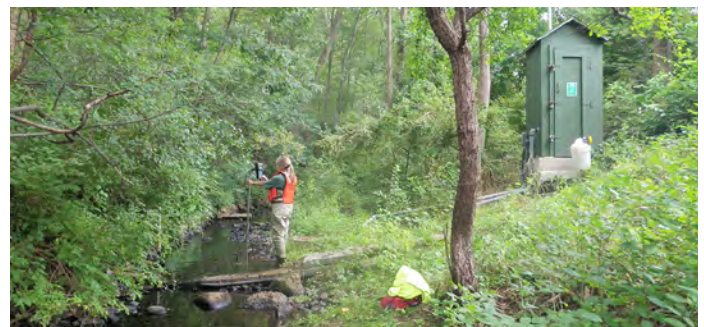
Discharge measurement at U.S. Geological Survey streamgage (01104415) near Lexington, Mass.
