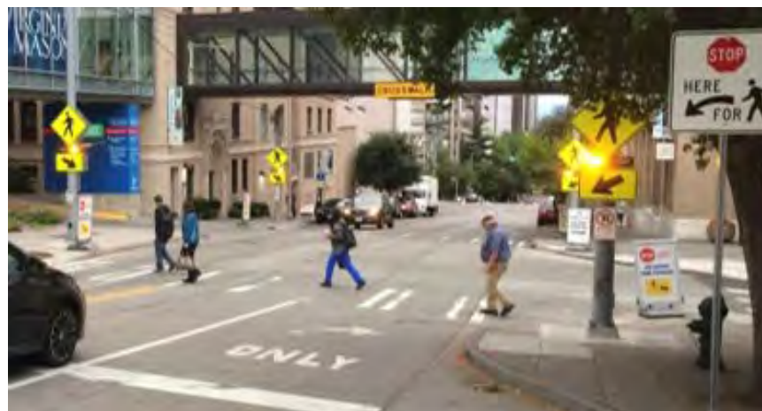
Rectangular Rapid Flashing Beacon (RRFB)
