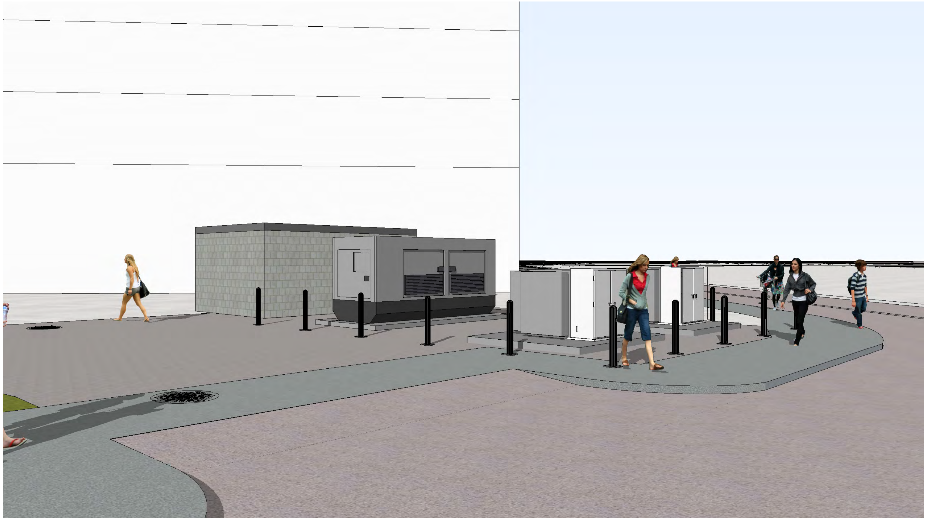
Precast concrete pump station building with no fence & trellis
