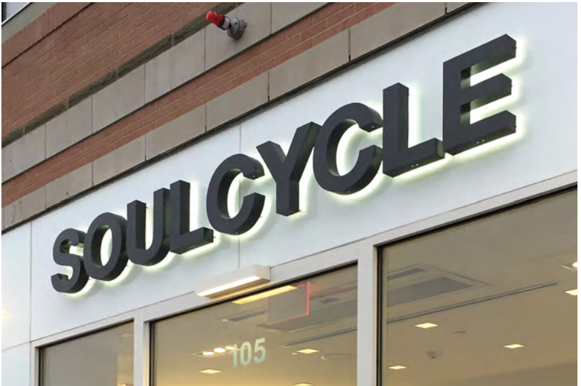
Preferred: Halo-illumination: individual reverse channel letters with lighting concealed inside the letter, casting light behind the letter against an opaque sign panel of wall surface.
