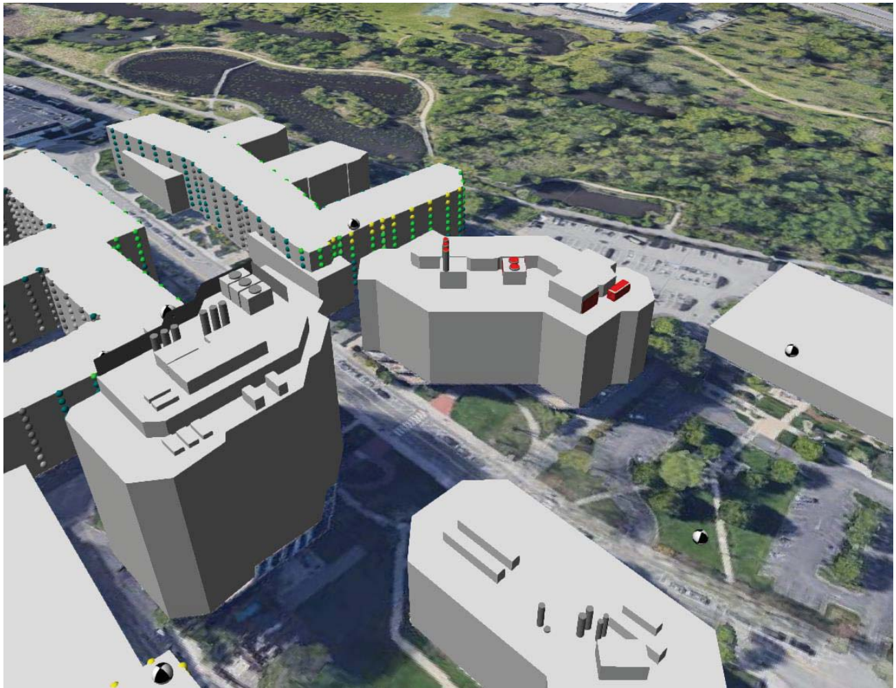
Figure 4 – “Bird’s-Eye” view of CadnaA noise model geometry, Phase 1
