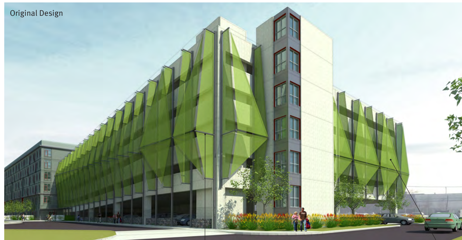
North Facade: Shape of banners changes across the length of the facade. Banners are mounted perpendicular to address the more oblique pedestrian approaches
