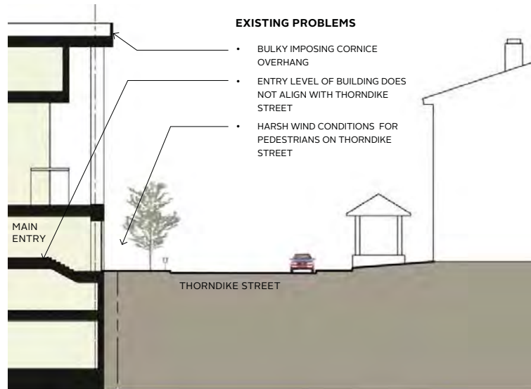
EXISTING SECTION THROUGH THORNDIKE STREET
