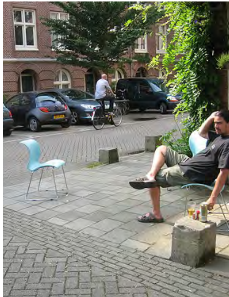
Above: A typical "Woonerf" in Europe. A Shared Street with no curb separation between cars, pedestrians, and bicyclists.
