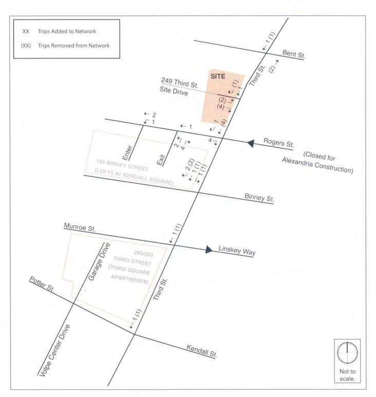
Figure 3.D.2 Project Relocated Trips - Lofts at Kendall Square, a.m. Peak Hour
