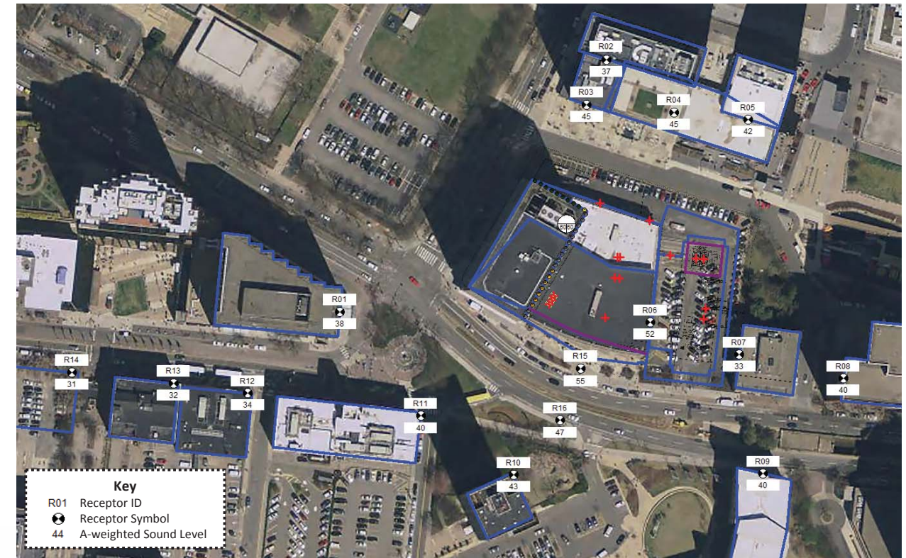
Kendall Square Cambridge – Predicted Daytime Noise from Outdoor Mechanical Equipment at One Broadway
