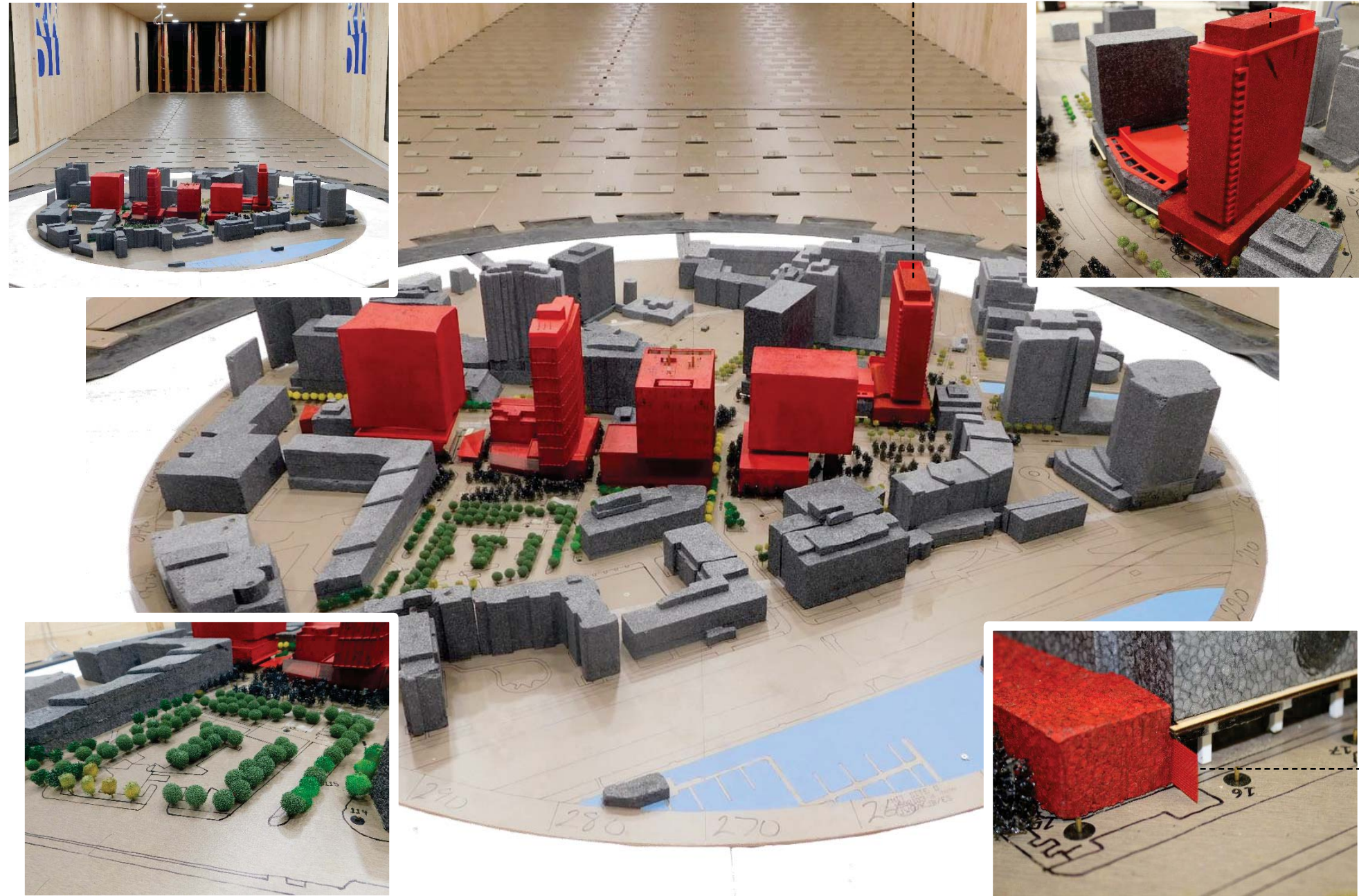
Wind Tunnel Study Model Full Build (NoMa and SoMa Tree Plans)
