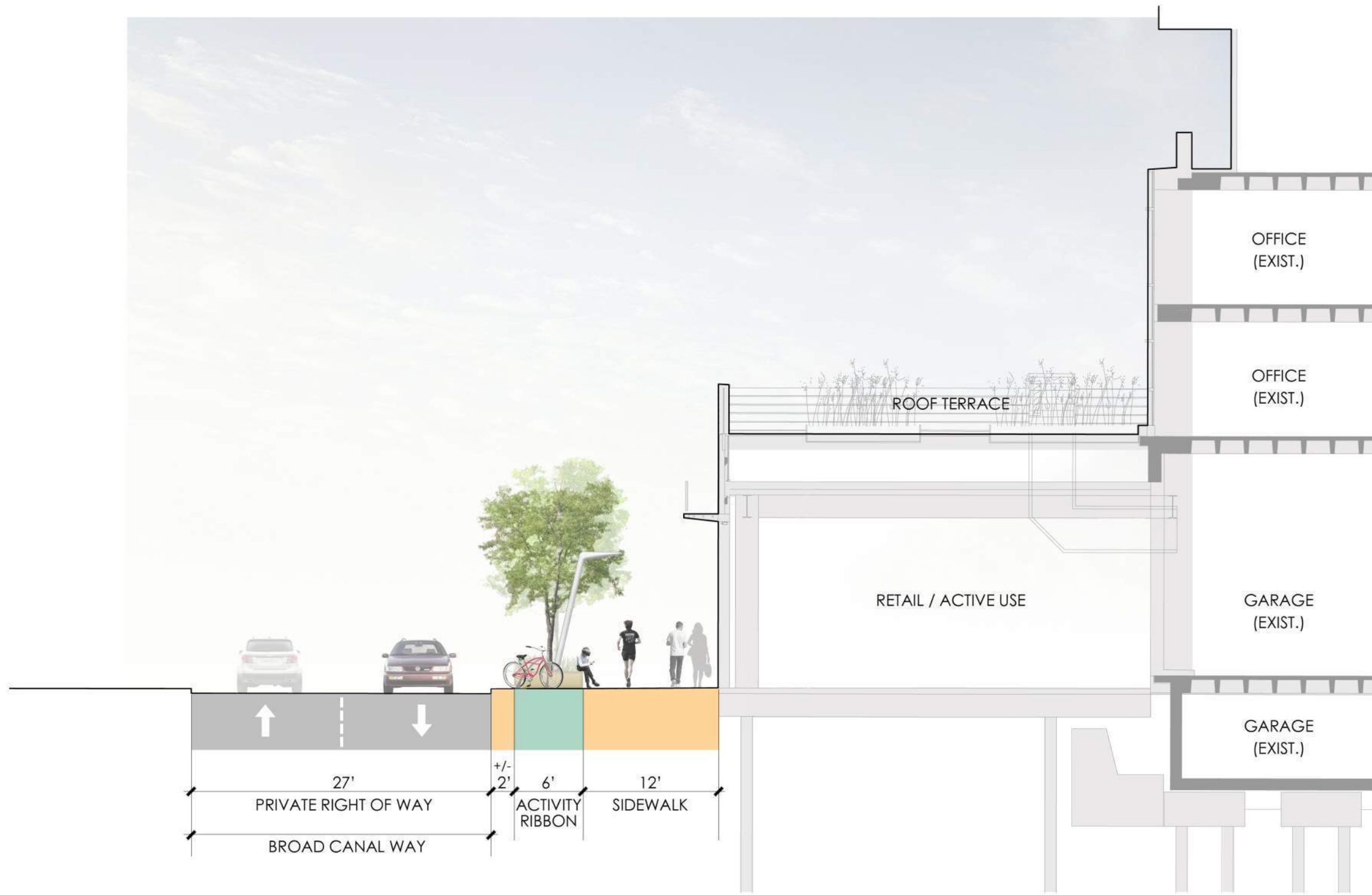
PROPOSED SECTION THROUGH BROAD CANAL WAY
