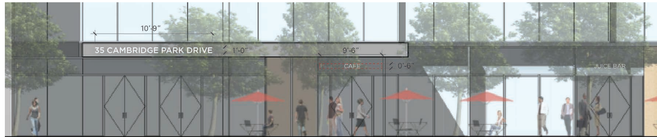
WALL SIGN BUILDING ID | ANCHOR TENANT SIGNAGE Dimensional acrylic lettering mounted to the face of entry canopy
