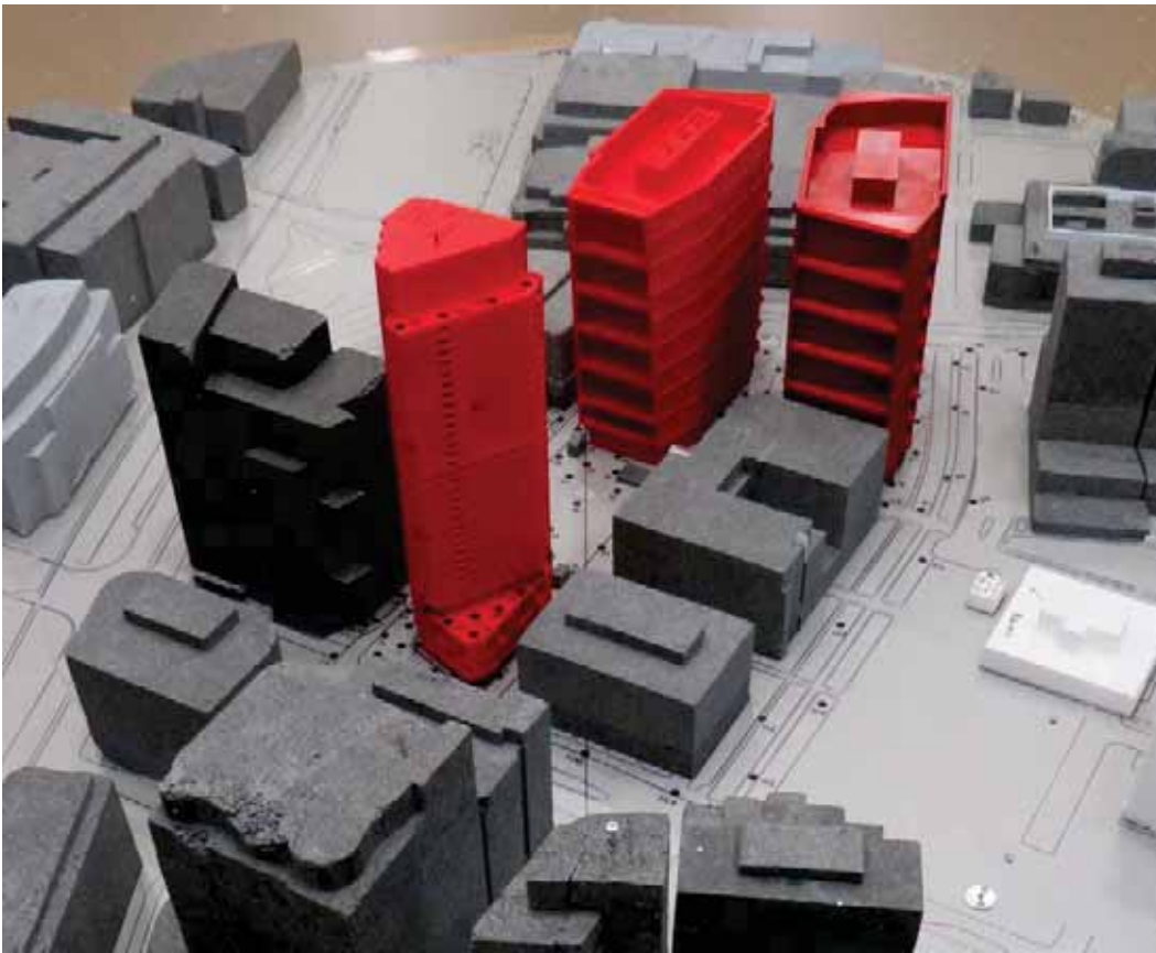
Image 4: Wind Tunnel Study Model – Proposed Configuration
