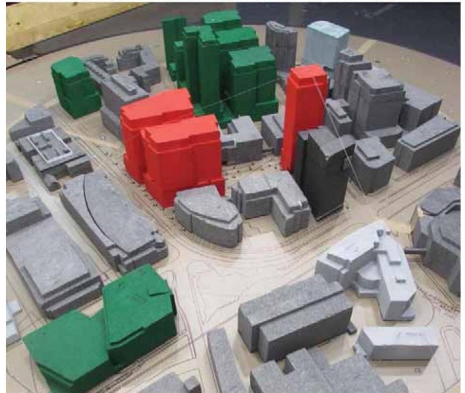
FIGURE 7.3C WIND TUNNEL STUDY MODEL - PROPOSED CONFIGURATION WITH VOLPE DEVELOPMENT
