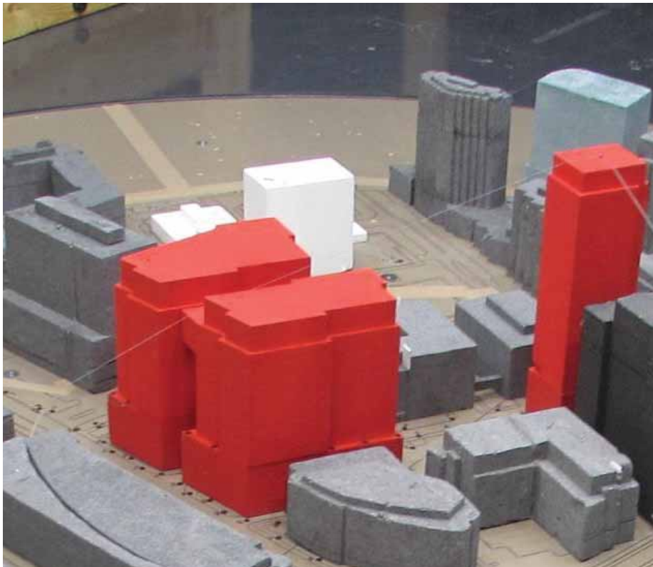
FIGURE 7.3B WIND TUNNEL STUDY MODEL - PROPOSED CONFIGURATION WITH GSA MASSING
